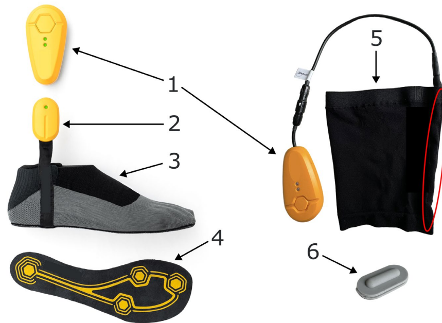
Figure 1. System components of the herein used vibrotactile feedback system (VTFS): (1) actuator unit, (2) transmitter unit, (3) sensor sock, (4) four pressure sensors at the heel, lateral midfoot area, medial midfoot area and big toe, (5) elastic leg cuff with the embedded vibration actuators (marked in red), (6) single vibration actuator (Copyright Saphenus Medical Technology GmbH).
