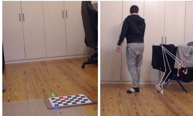
Figure 5.3: Checkerboard pattern with visualized world coordinate system axes (left), and (right) an example of MediaPipe’s pose detection failure case where the algorithm incorrectly detected human pose keypoints on a drawer instead of the actual person in the scene.
