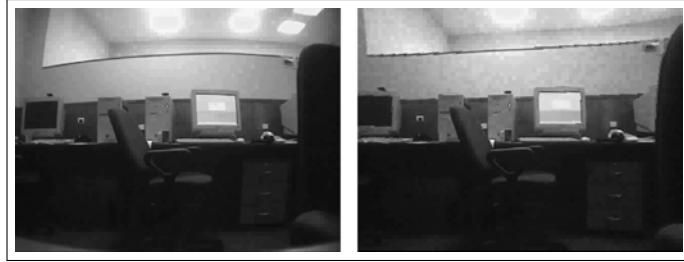
Figure 2.5: Camera image before undistortion (left) and after (right). Source: Bradski and Kaehler, Learning OpenCV [9, p. 678]
