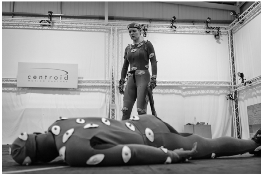
Figure 2.1: Optical motion capture (mocap)—actors wearing mocap suits with reflectors Source: Achrekar, A. In [17, p. 12]. Courtesy of Centroid Motion Capture.
