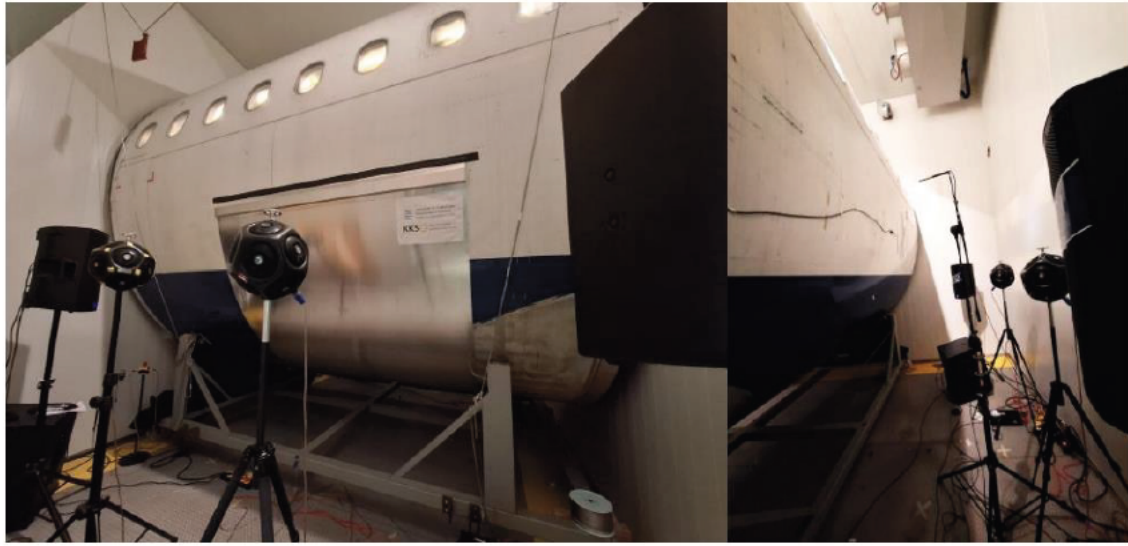
Figure 22: Experimental set-up with 4 dodecahedron speakers, 2 IQ12 speakers and 2 speakers [31]
