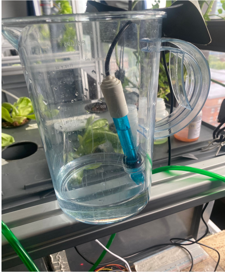
Figure 41: Calibration was done periodically for a week, with liquids of different pHs
