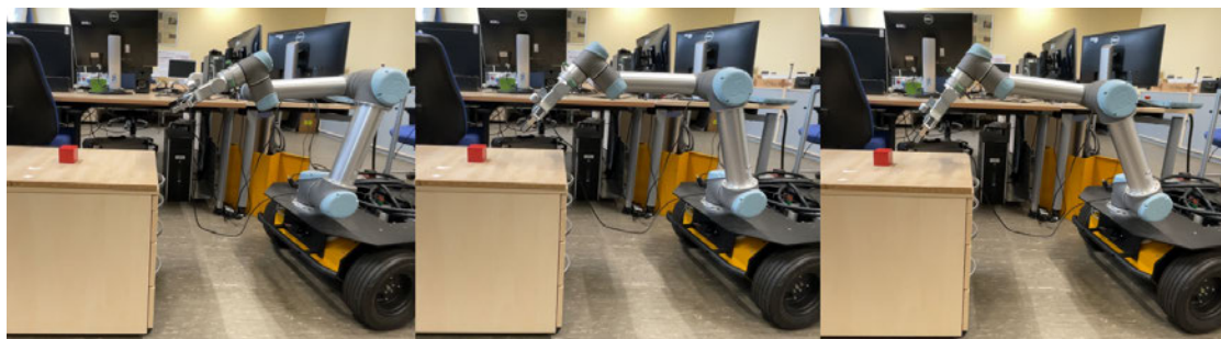
Figure 5.15: First transfer of the policy to the real domain after a successful validation run in the simulation. The image on the right shows the tool stalling without initiating the grasp.
