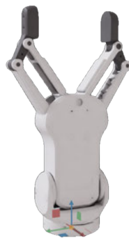
Figure 4.6: RG6 two finger gripper imported via IsaacSim and adapted from the URDF.
