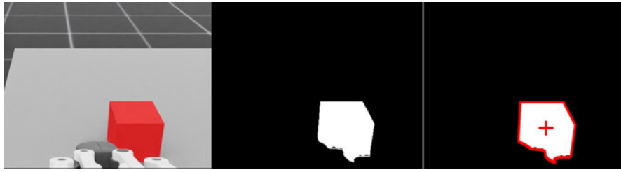
Figure 4.2: Main three steps of the cube detection and centroid position calculation process illustrated from left to right.
