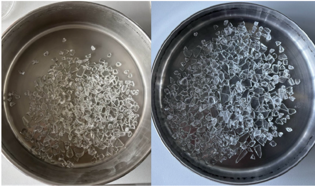
Figure 34: Cutting-milled glass sample with 20mm sieve, batch 1 (left) and batch 2 (right) (author's own photograph).
