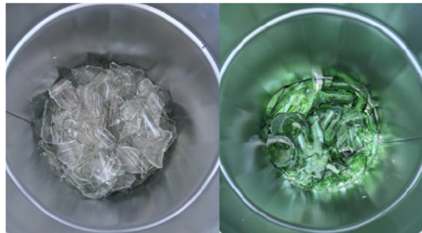
Figure 24: clear (left) and green (right) glass samples after manual hammer crushing (author's own photograph).
