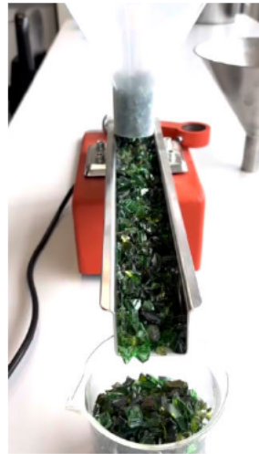
Figure 23: Glass particles in the vibrating chute prototype (author's own photograph).
