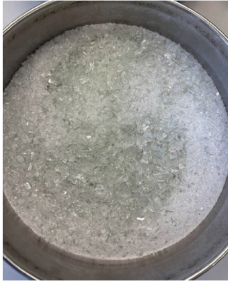
Figure 30: Jaw-crushed glass sample at 5 mm jaw gap (author's own photograph).
