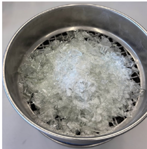
Figure 29: Jaw-crushed glass sample at 2,5 mm jaw gap (author's own photograph).
