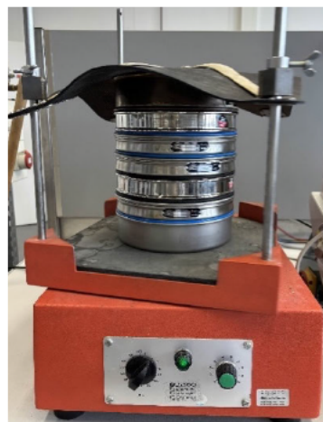
Figure 18: Sieving tower from Fritsch GmbH, HAW Hamburg (author's own photograph).
