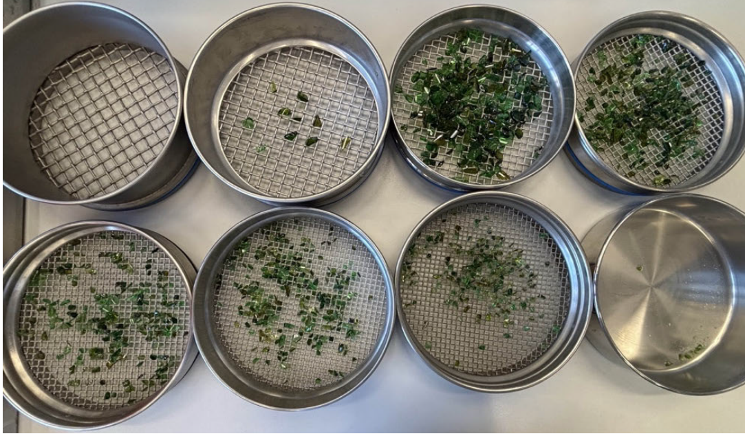
Figure 38: Green glass sample according to DIN (author's own photograph).
