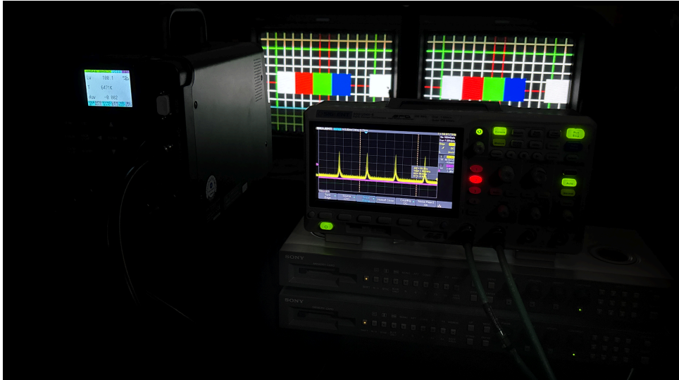
Figure 12: Alignment setup for measuring CRT displays, locking the spectroradiometer to the light output is done with a photodiode and an Oscilloscope.
