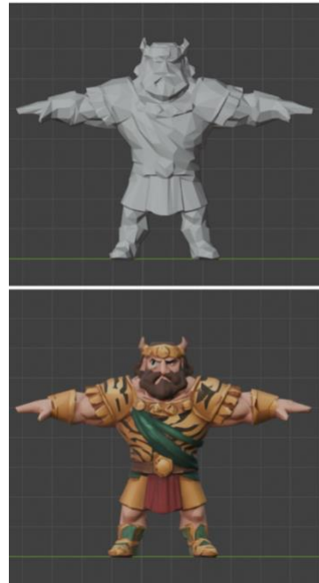
Figure 17: Manually optimized low-polygon model created by decimating a high-polygon mesh in Blender..
