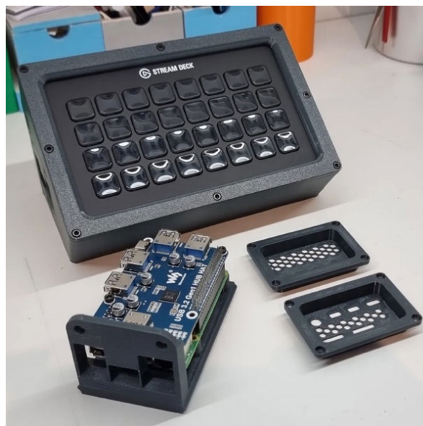
Abbildung 25: Stream Deck XL-Companion-Pi-Setup. Quelle: Atelier Du Tech (2024).
