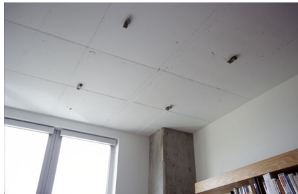
Abbildung 3.2.: Cricket Beacons an der Decke montiert [MIT Computer Science and Artificial Intelligence Lab Cambridge, MA 02139 (2005b)]
