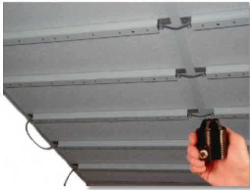
Abbildung 3.6.: HiBall Beacon Array [3rdtech (2010b)]
