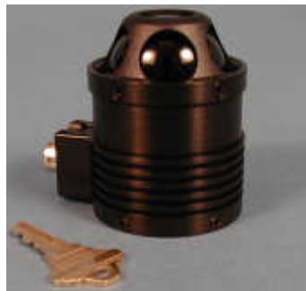
Abbildung 3.7.: HiBall Sensor [3rdtech (2010c)]
