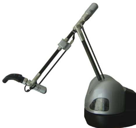
Figure 2.10: Ground-referenced haptic display from Haption 9
