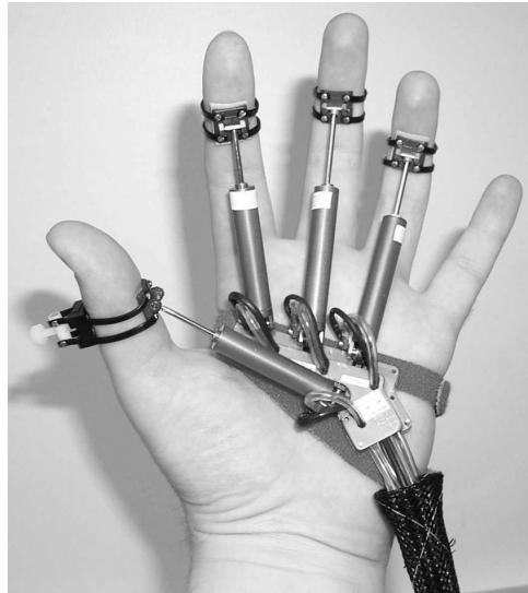
Figure 2.11: Body-referenced haptic display [2]
