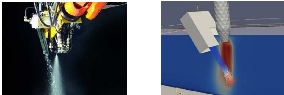
Figure 1.1: PUR-CSM Process (© Hennecke GmbH) (Left) and Simulation of Fiber Spray Process (Right)
