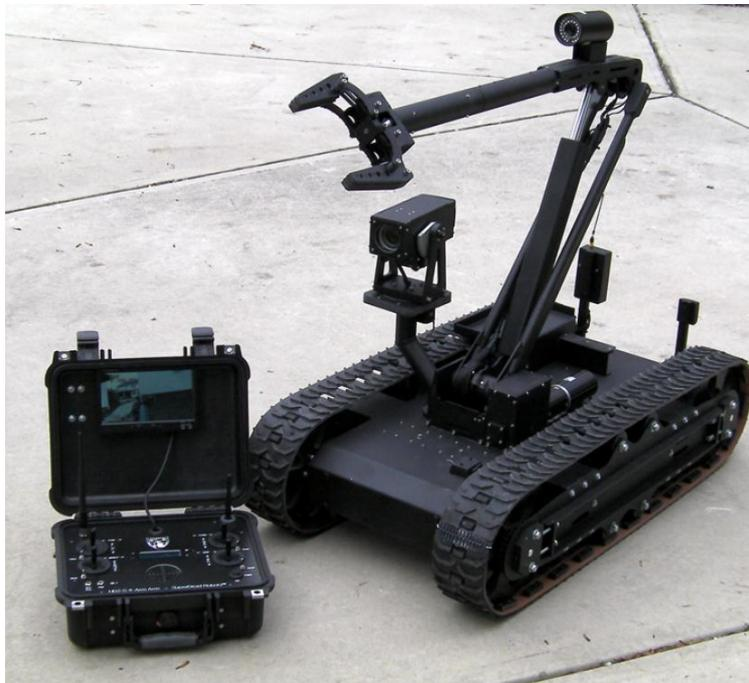
Abbildung 2-3 HD2 SWAT / EOD Tactical Treaded Robot, Bild © 2010 SuperDroid
