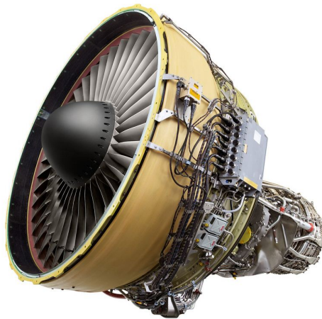
Figure 1.1: General Electric CF6-80C2 [GE10]
