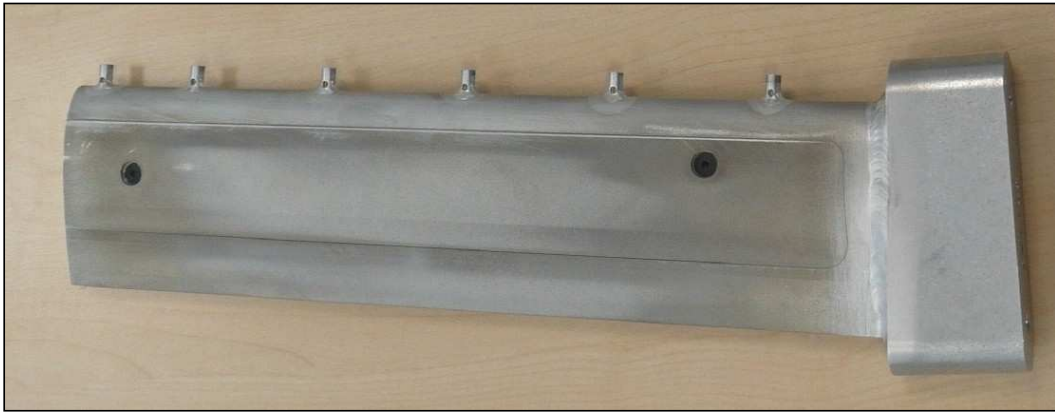
Figure 7.4: Rake for temperature and pressure measurement
