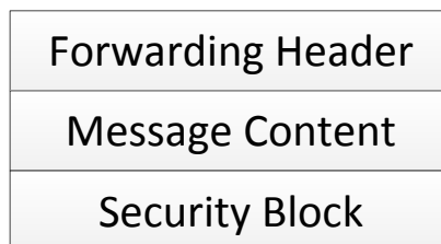
Figure 9: Structure: Composition of a RELOAD message
