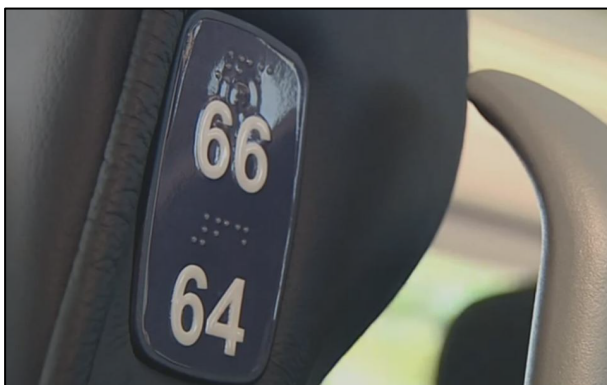
Figure 32: Tactile seat numbers with Braille [43]
