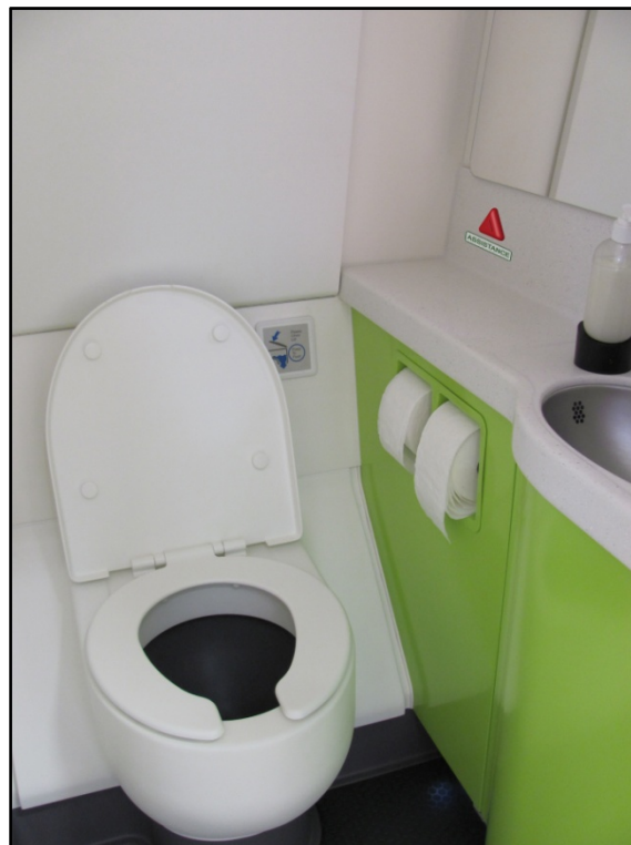
Figure 63: Location of the modified attendant call button and placard inside an A320 lavatory [Source: Author]
