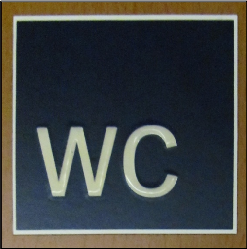
Figure 35: Tactile placard on the ICE lavatory door [Source: Author]
