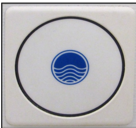
Figure 58: Flush button inside an A380 [Source: Author]
