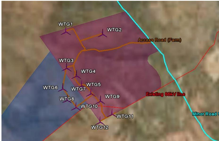
Figure 1 Simplified Site Layout including Property Boundaries, Turbine Positions and planned Access and Turbine Roads
