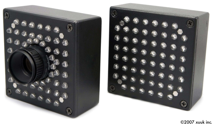
Abbildung 4.5: Links: Kamera, Rechts: Illuminator
