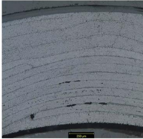
Figure 2.6.2- 2 Voids in the interlayer region at the ply-drop
