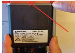
7. Secure the module by inserting the sealable red locking strap provided for this purpose.
