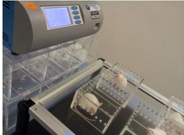
**Figure 11** Hargreaves control unit, acrylic chambers and glass table
