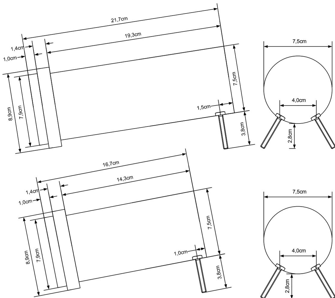
**Figure 14 Measurements of burrowing devices**
