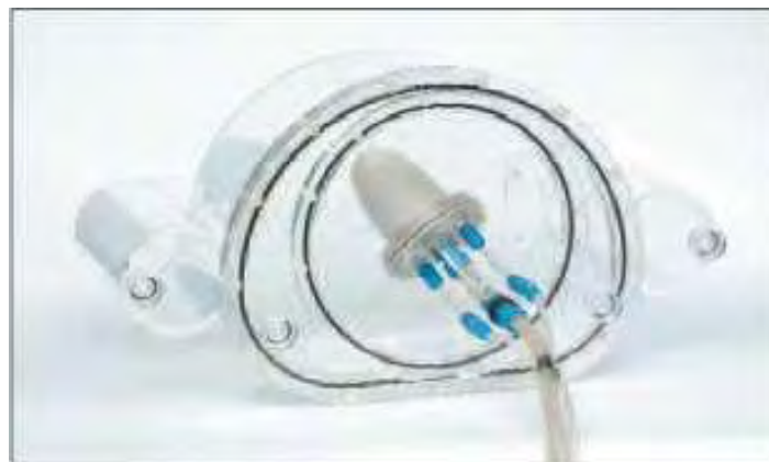
Figure 2.1 Dynamic cardiac phantom simulating left ventricle , capable of operating at 60 bpm (19).
