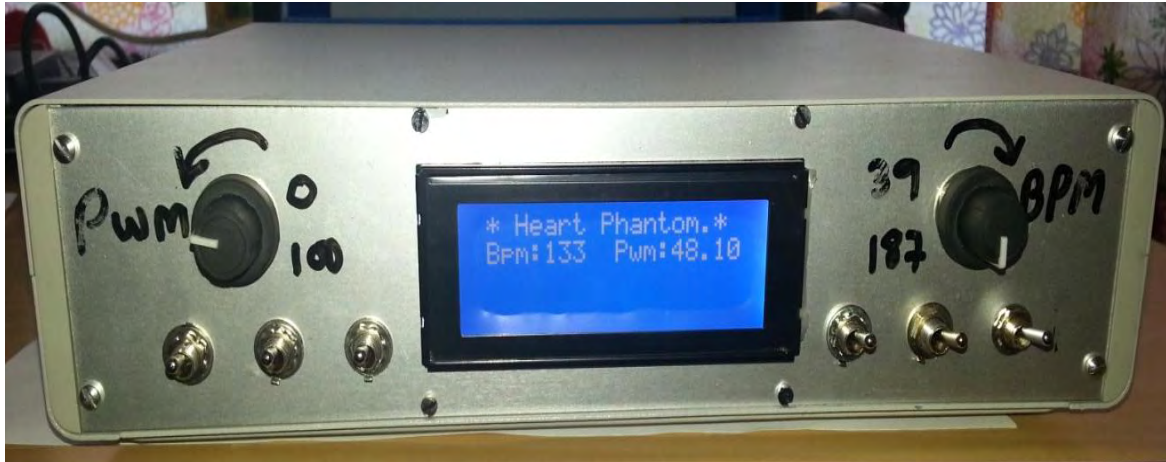
Figure 4.10 view of the control box. 6 Rocker switch for controlling V.P. and S.V.. Two potentiometers for pulse width and Front frequency control.
