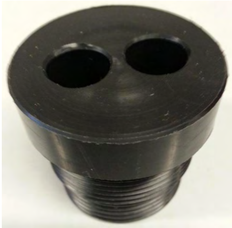
Figure 4.6 Balloon holder with two Ø12mm holes for holding valves or connecting silicone pipes.
