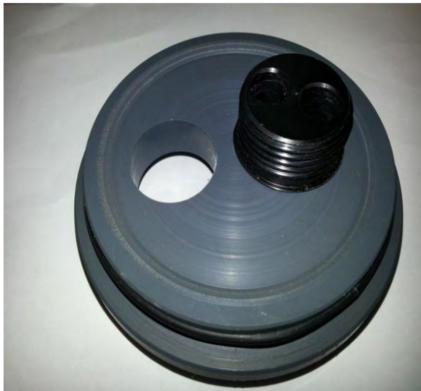
Figure 4.7 Balloon holder fitted on top cover
