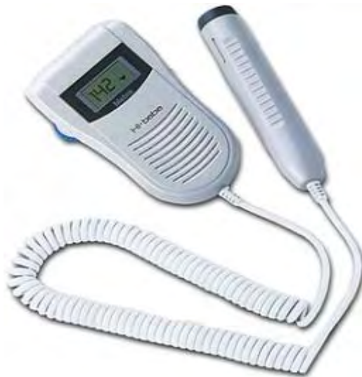
Figure 3.9 Single element hand-held portable Doppler device (32).
