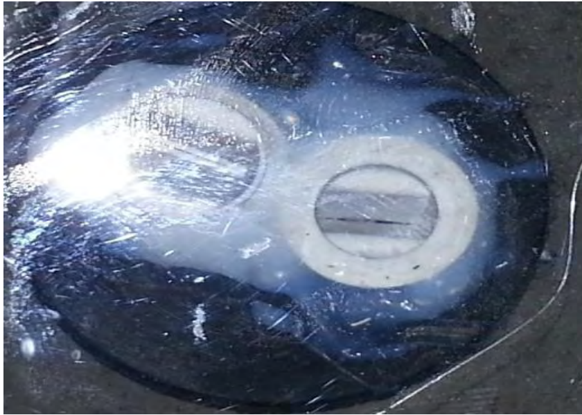
Figure 4.8 Holder with two uni-directional valves facing opposite direction
