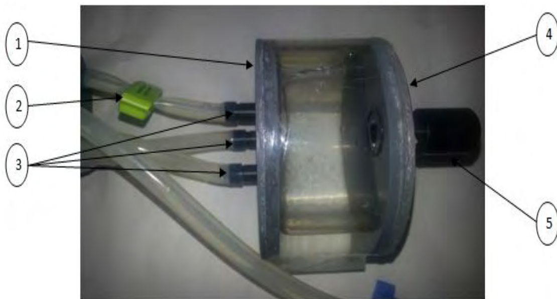
Figure 4.3 Reservoir chamber filled water, It has a top opening and three bottom opening for connection with ventricular chamber using silicone pipes.
