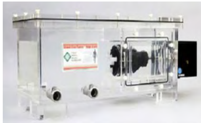
Figure 2.3 Dynamic heart phantom for multi-modal testing (22). Capable of operating at 200 beats per minute.
