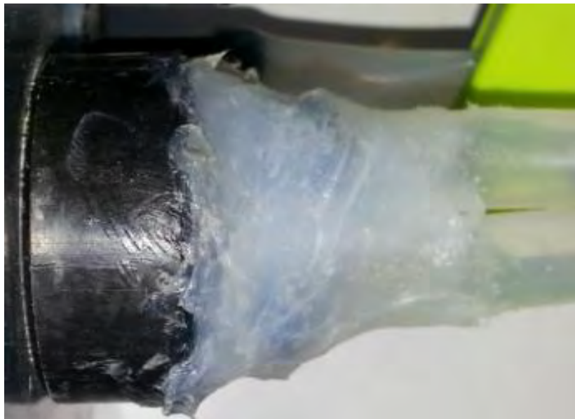
Figure 4.9 Holder with two Ø8mm silicone tubes fitted and covered with silicone glue.
