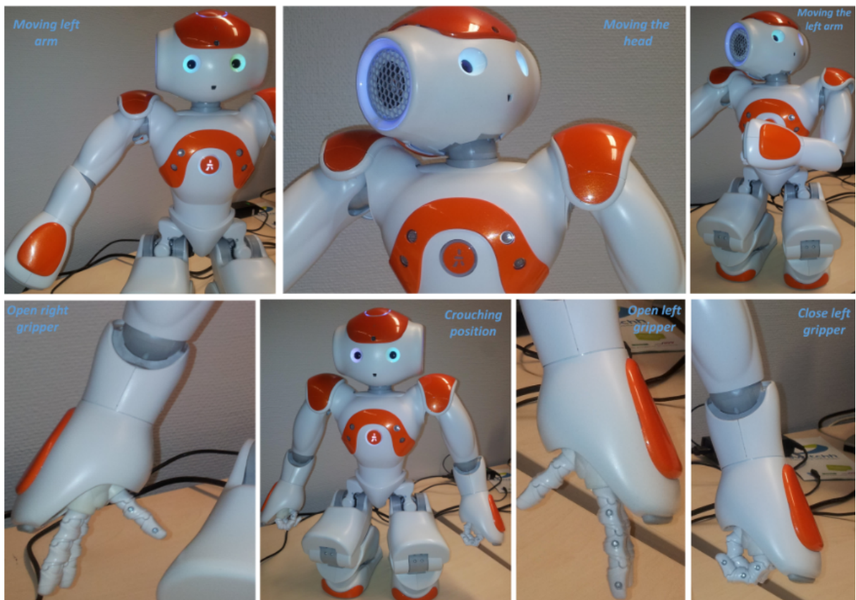
Figure 6.3: Experiments to manipulate the Nao robot
