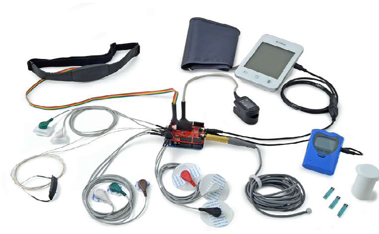
Figure 49: e-Health Sensor Platform V2.0 connected with various medical equipment to visualize the possibilities (source: www.cooking-hacks.com , (the open hardware division of Libelium))
