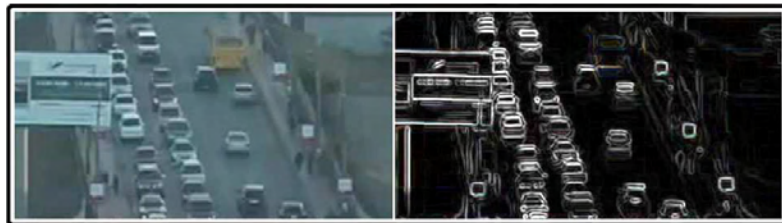
Figure 28: Comparison of the original image (left) with a calculated image of an easy edge detection algorithm (right). The original camera image is from the YouTube movie: "Ulaanbaatar - Metro tusiin taniitsuulga"
