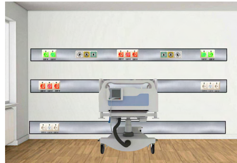
Figure 25: Design concept for the ICU at the National Central Hospital. "Schuko" 220 Volt and Nema 5-15P 110 Volt sockets in white, orange and green colours for their specific purposes.
