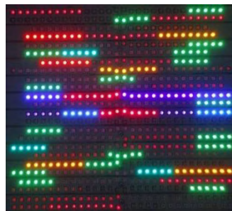
Figure 4.1: LED Array used in the solar simulator
