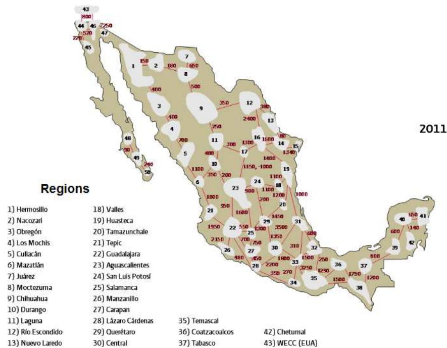
Figure 4 Map of the main transmission lines in Mexico. Circled is the id number of each transmission line and over the lines its capacity.
