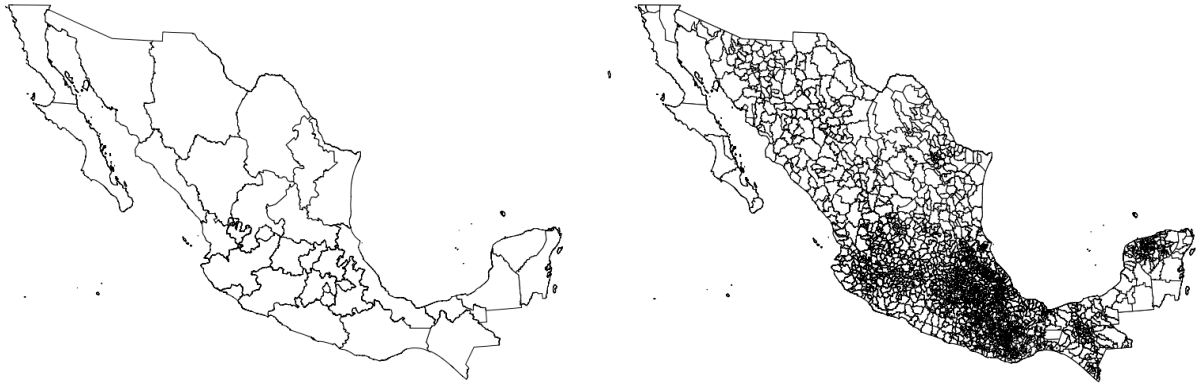
Figure 30 First maps obtained by INEGI. The one on the left represents the states and the one on the right the municipalities of the country. From the map of the left, the states had to be extracted and then merged with the map of the right to obtain the municipalities in the State. Around 400 maps had to be created
