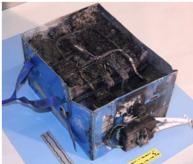
Abb. 23: Zerstörte Li-Batterie des Dreamliners (National Transportation Safety Board, 2014)
