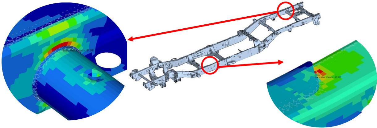
Figure 5-8: Locations for the maximum stresses during both loadcases
