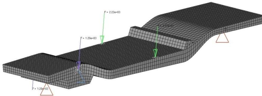
Figure 6-2: FE model which defines the frame's space
