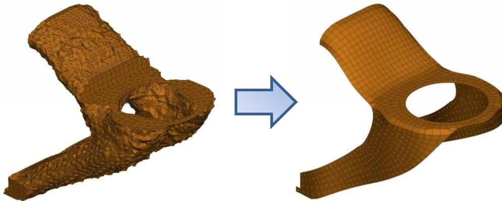
Figure 8-9: Modeling the topology result to a FE model
