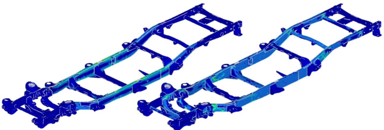
Figure 6-10: Gauge optimization: Stresses for static loadcases
