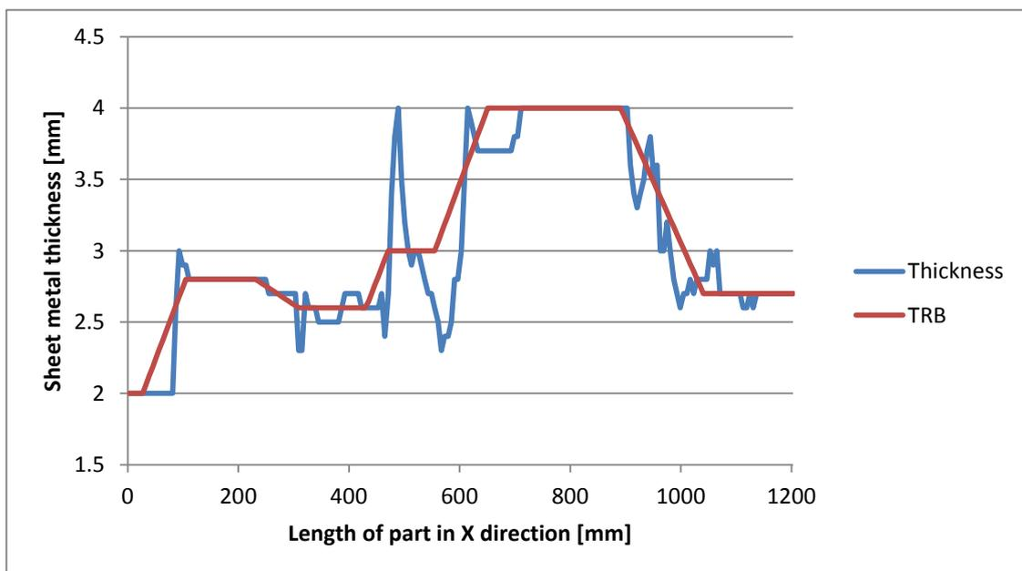
Figure 6-39: Thickness Distribution Before and after the manual FE design
