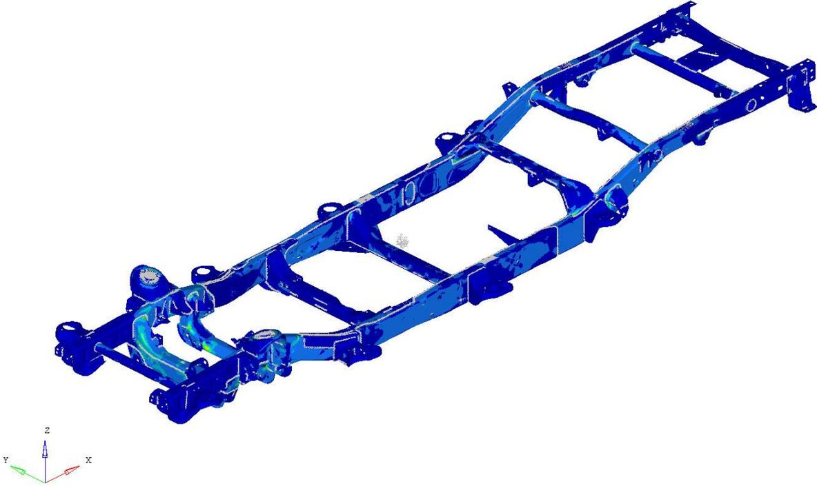
Figure A-8: Aluminum result: Von Mises stress for torsion LC
