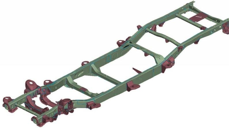
Figure 6-18: Material optimization: Part selection for whole aluminum body
