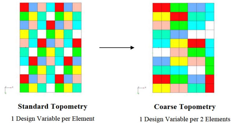
Figure 6-29: Difference between topometry and coarse topometry [29]
