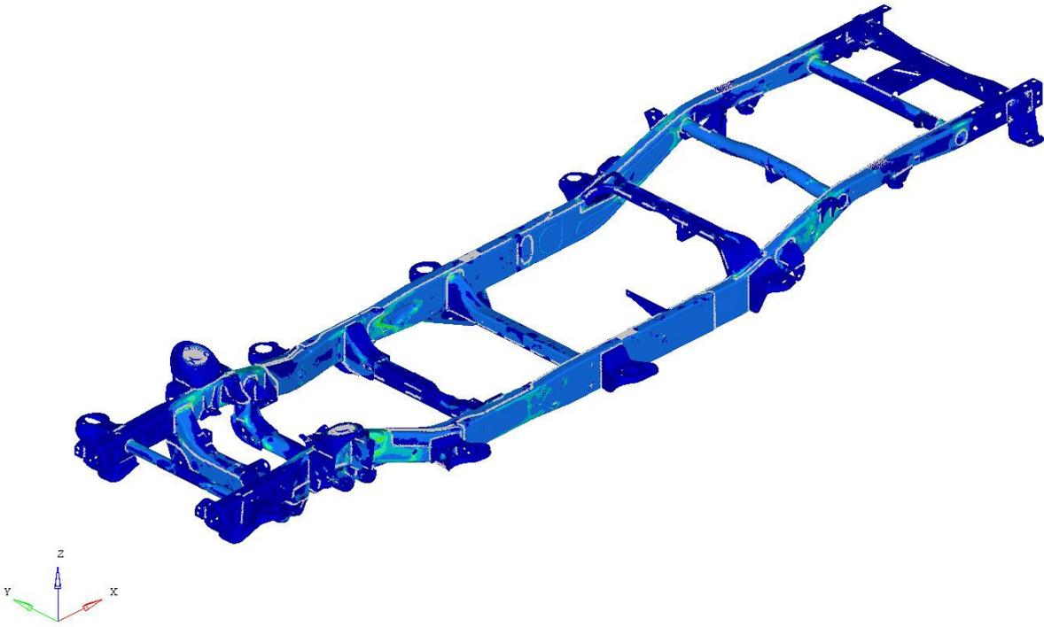
Figure A-4: Gauge result: Von Mises stress for torsion LC
