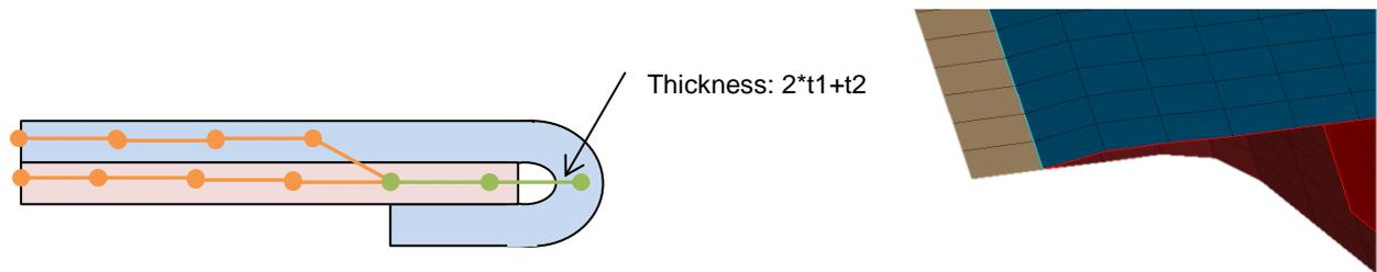
Figure 5-5: Recommended way to mesh hems
