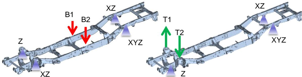
Figure 5-7: Locations for loads and constraints
