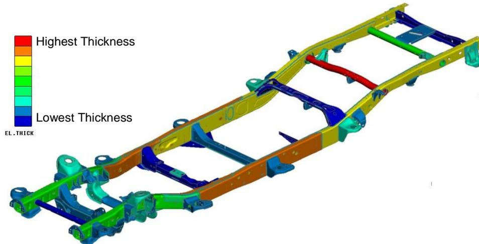
Figure 6-23: Material optimization: Thickness overview (Aluminum frame)
