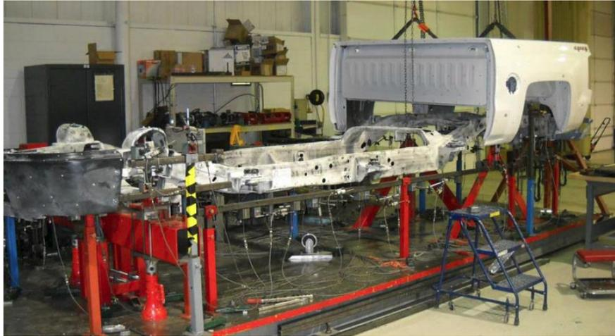
Figure 5-1: Test setup for static tests
