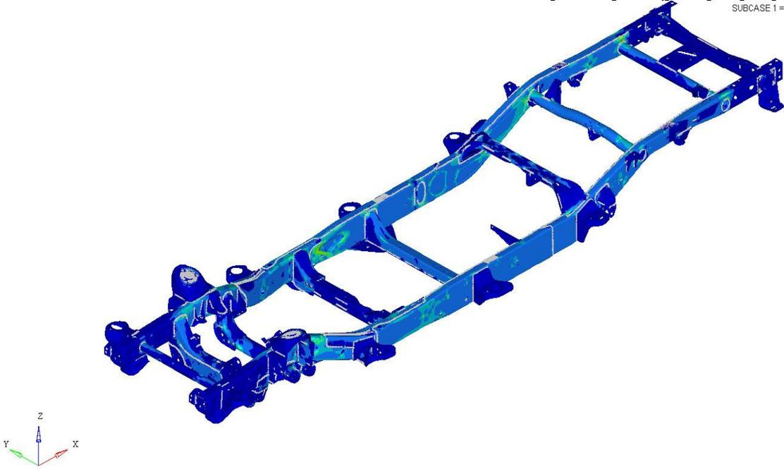
Figure A-2: Baseline result: Von Mises stress for torsion LC
