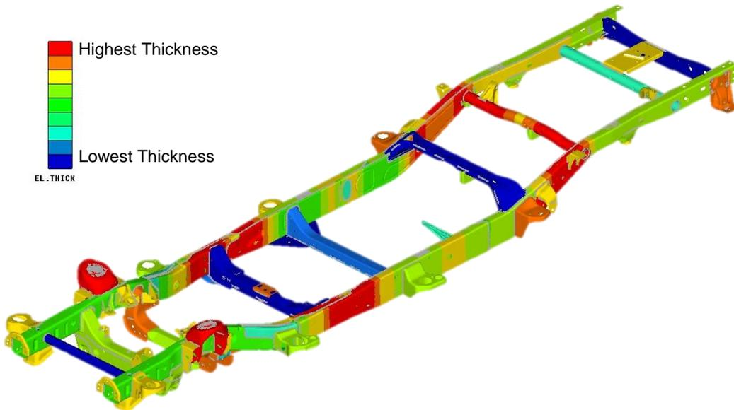
Figure 6-41: Semi-manual TRB: Thickness Overview
