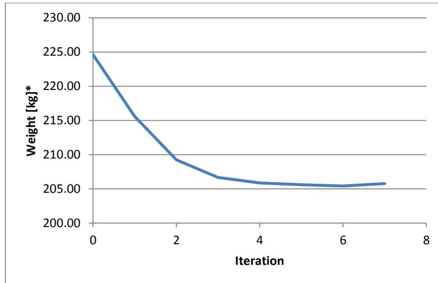
Figure 6-8: Gauge optimization: Objective vs. Iteration
