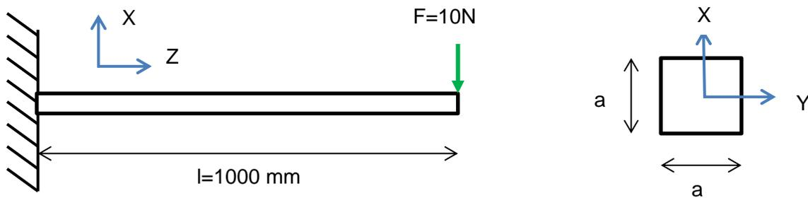
Figure 6-11: Example problem: Beam with bending force
