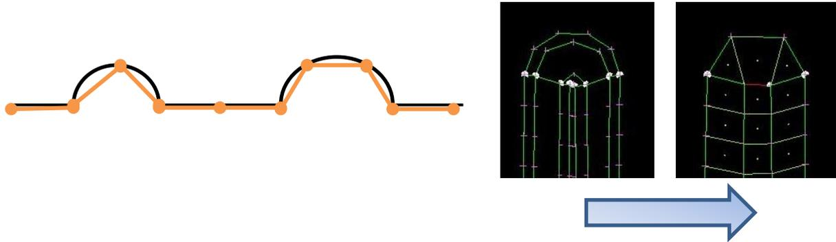
Figure 5-3: Recommended way to mesh beads
