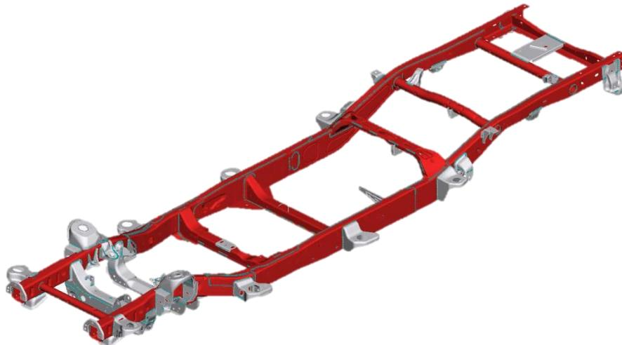
Figure 6-7: Selected parts for gauge optimization
