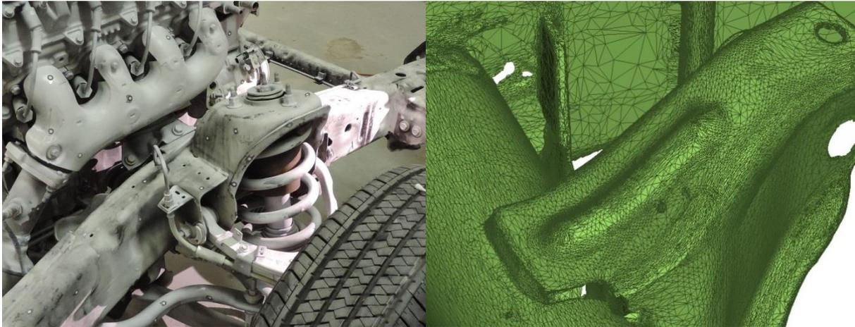
Figure 5-2: Prepared frame before the scan; digitalized scan
