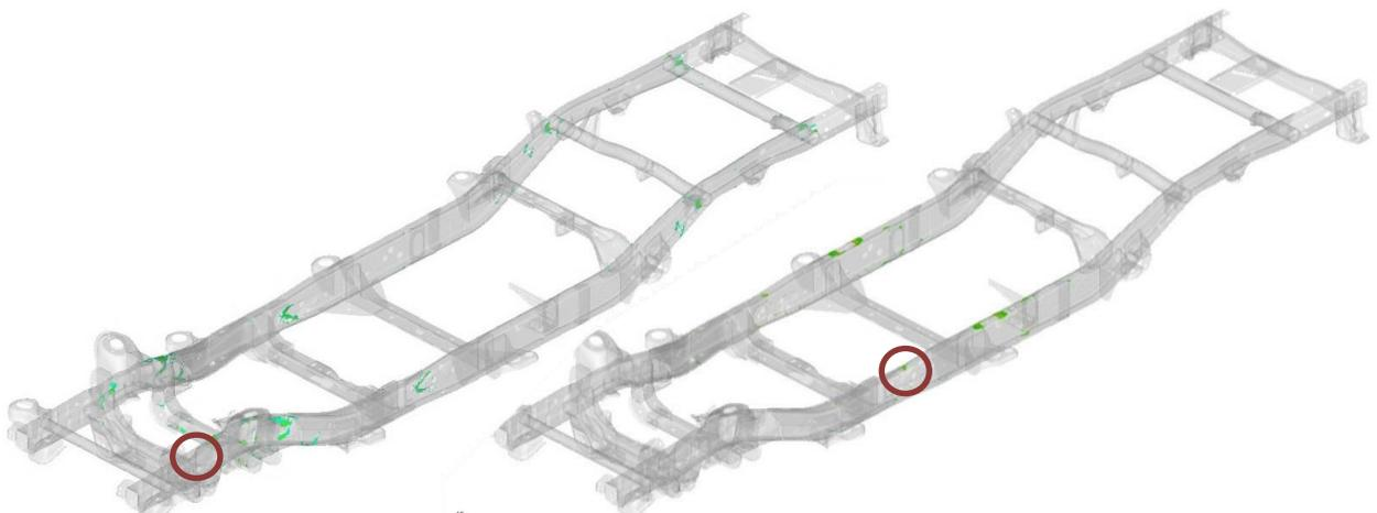
Figure 6-17: Material optimization: Von Mises stresses over 25 MPa
