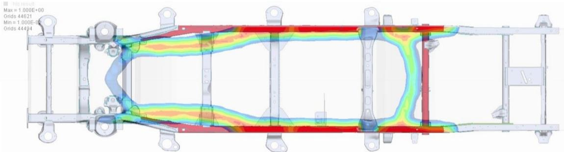
Figure 6-27: Topometry optimization: Merged topological result with frame
