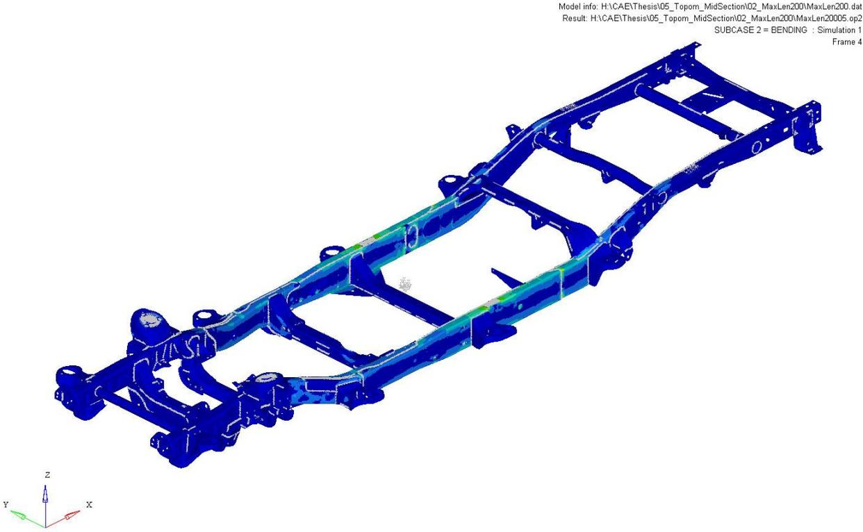
Figure A-9: TWB 200 mm width result: Von Mises stress for bending LC
