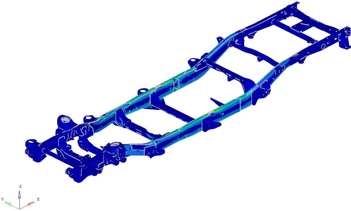
Figure A-3: Gauge result: Von Mises stress for bending LC
