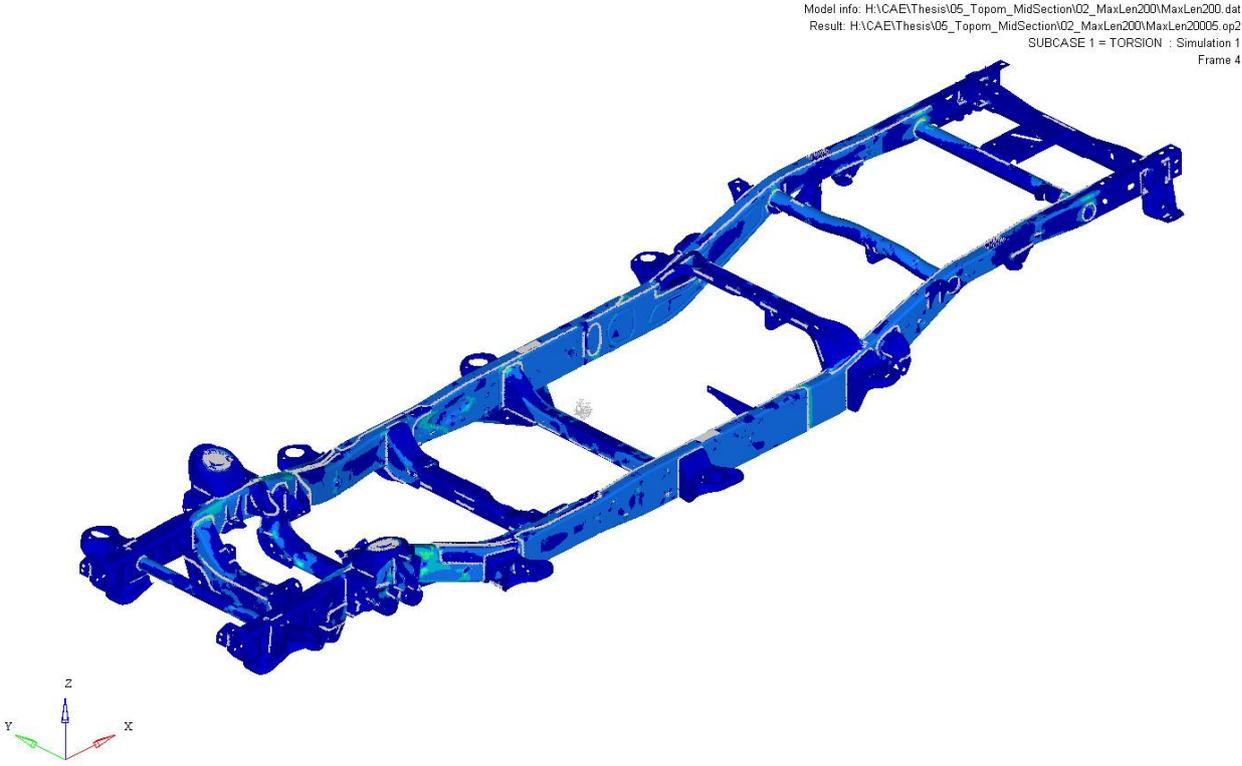
Figure A-10: TWB 200 mm width result: Von Mises stress for torsion LC
