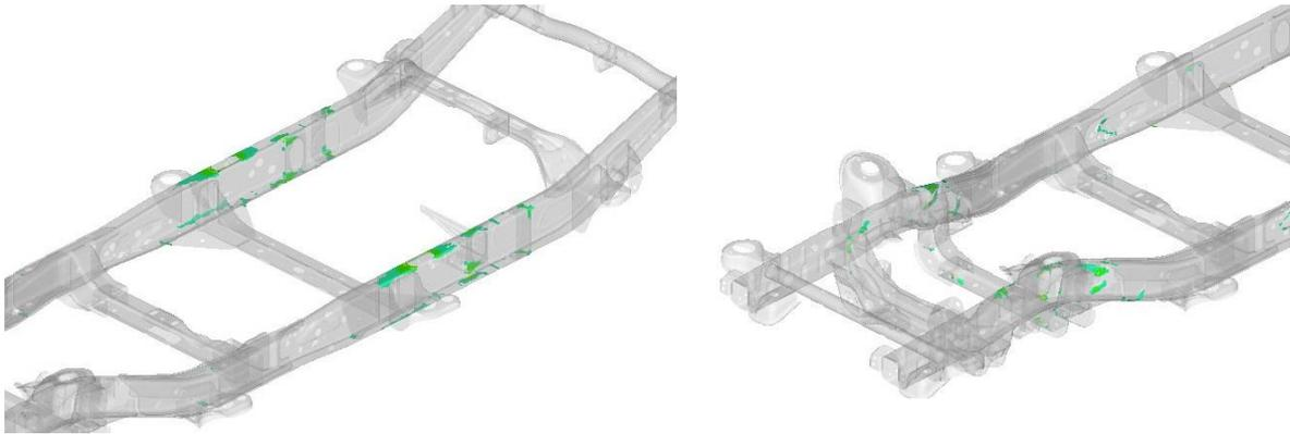
Figure 6-37: Semi-manual TWB: Von Mises stresses over 25 MPa
