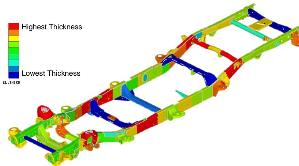
Figure 6-38: Semi-manual TWB: Thickness overview
