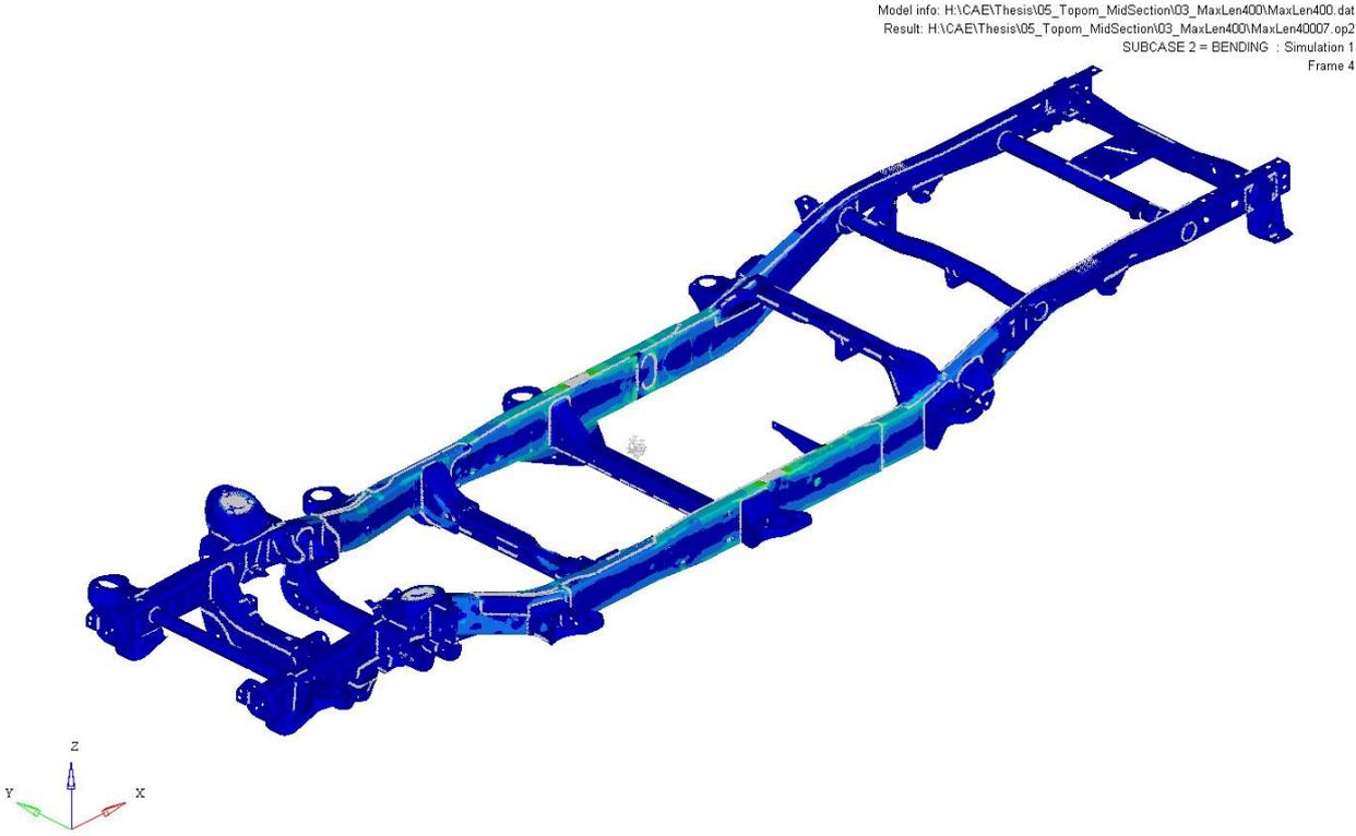
Figure A-11: TWB 400 mm width result: Von Mises stress for bending LC
