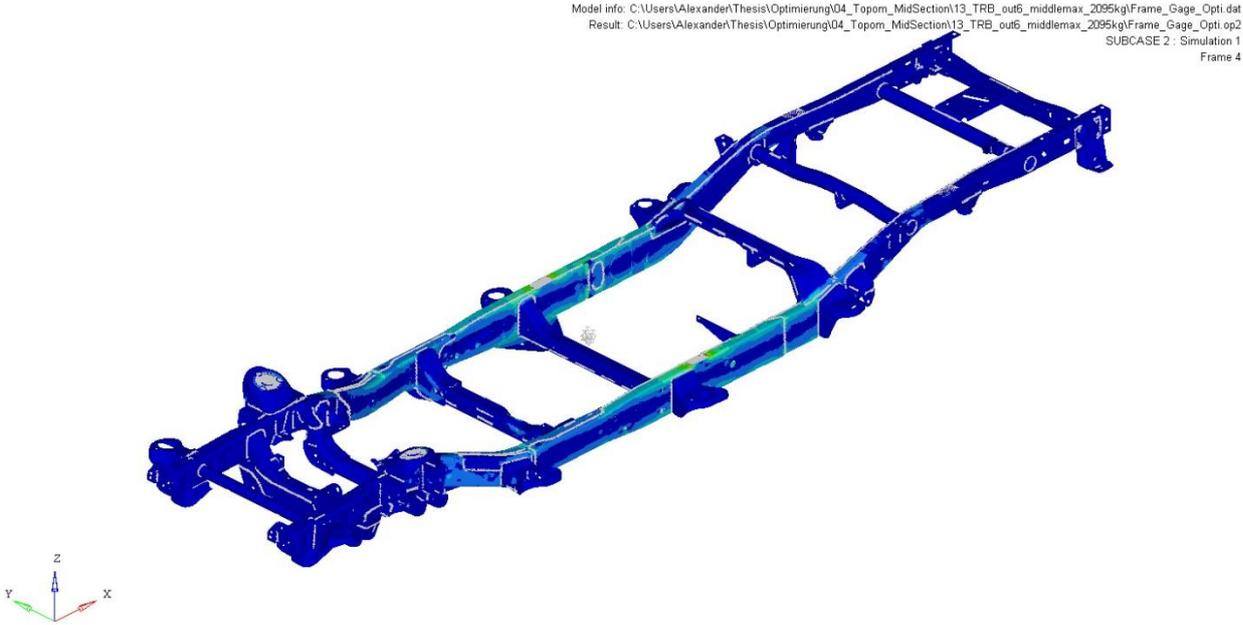
Figure A-15: Semi-manual TRB result: Von Mises stress for bending LC
