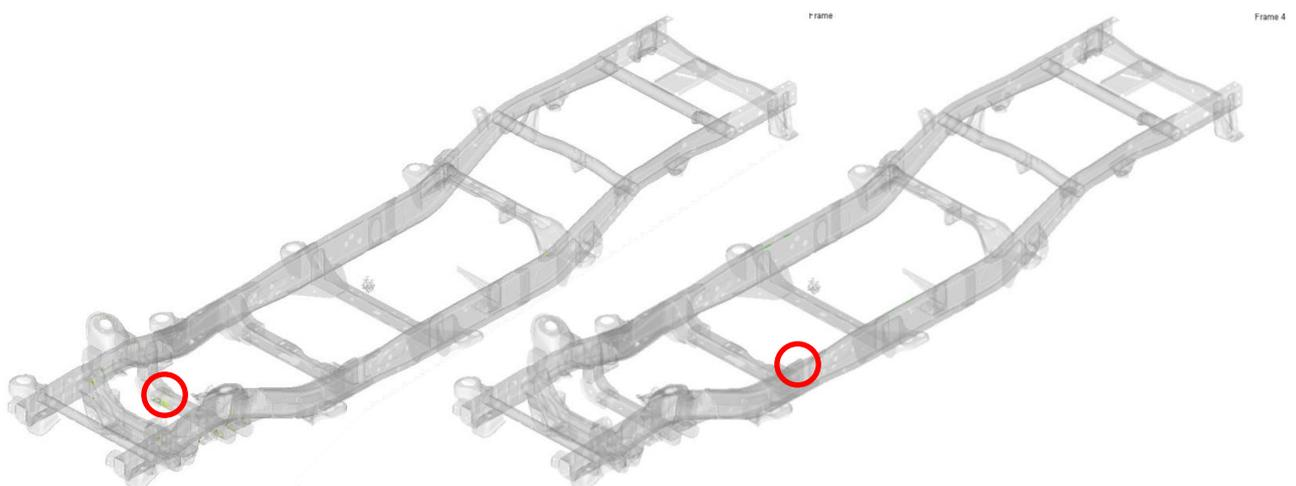
Figure 6-22: Material optimization: Von Mises stresses over 25 MPa (Aluminum frame)
