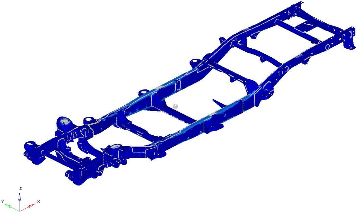
Figure A-7: Aluminum result: Von Mises stress for bending LC
