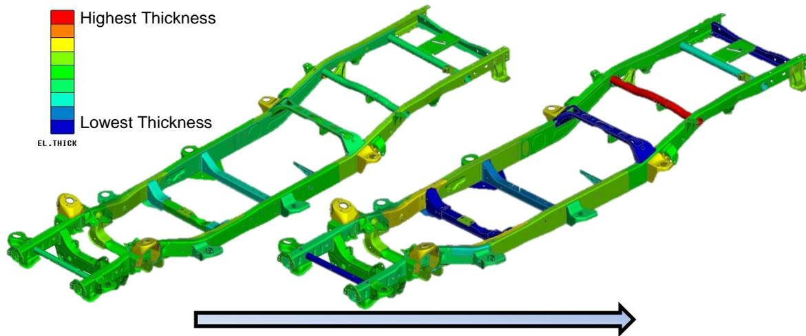
Figure 6-9: Gauge optimization: Changes for thickness
