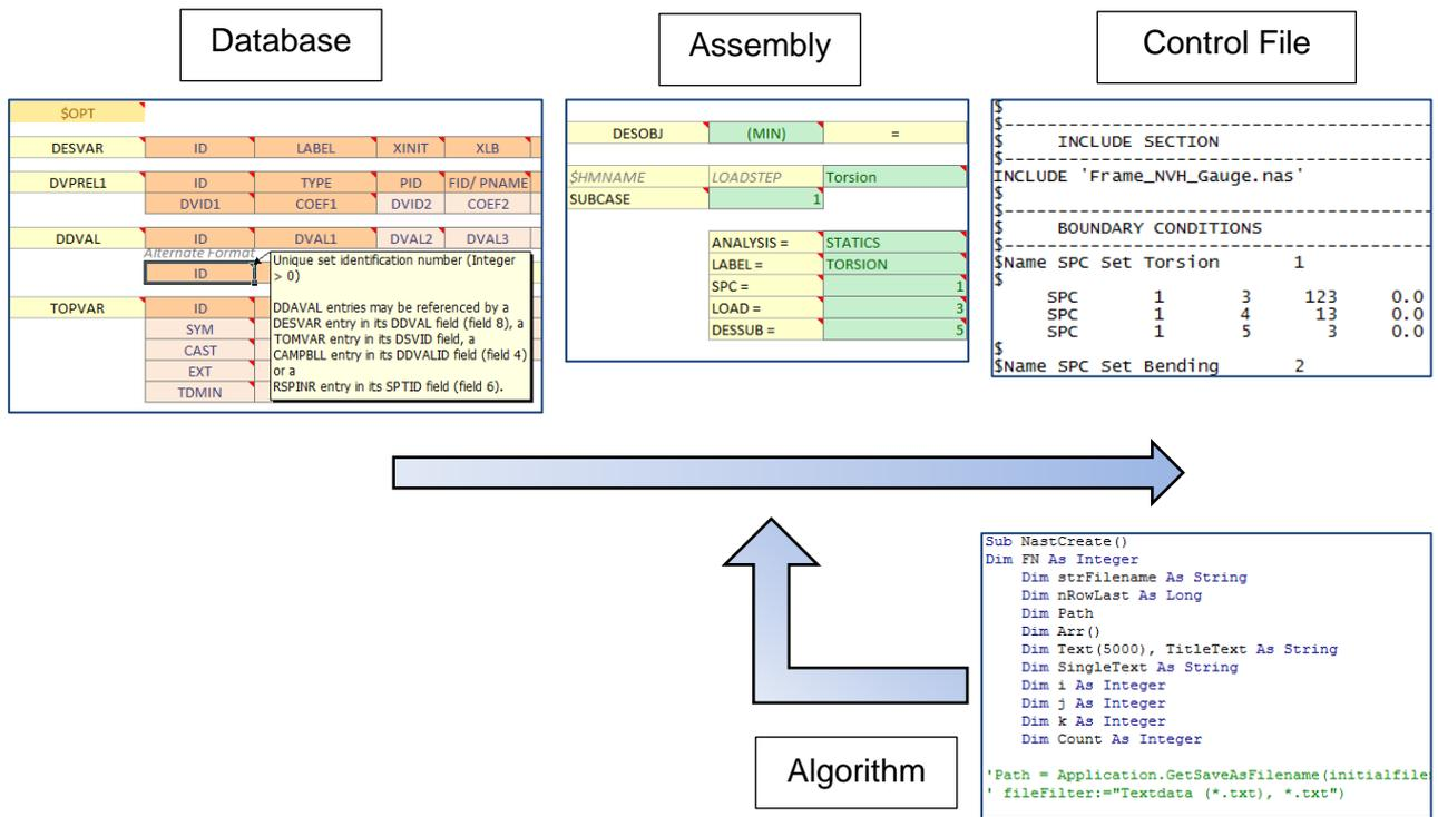
Figure 6-6: Work flow using the Excel Nastran SOL 200 Editor
