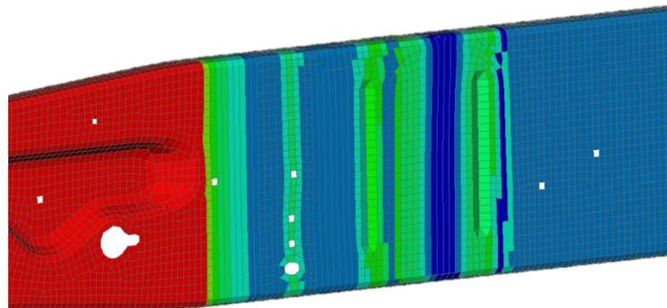
Figure 6-35: Semi-manual TWB: A region that will be merged to one blank
