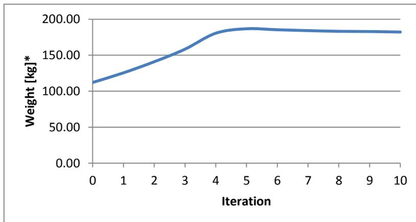
Figure 6-20: Material optimization: Objective vs. Iteration for whole aluminum frame
