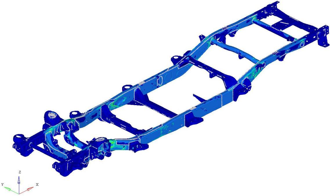
Figure A-6: Aluminum crossmembers result: Von Mises stress for torsion LC
