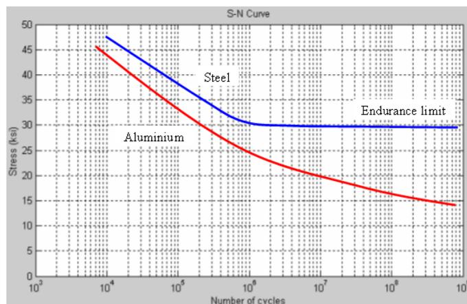
Figure 6-24: Stress vs. Number of cycles for aluminum and steel [28]
