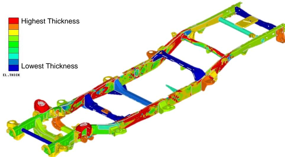
Figure 6-28: Topometry optimization: Thickness distribution
