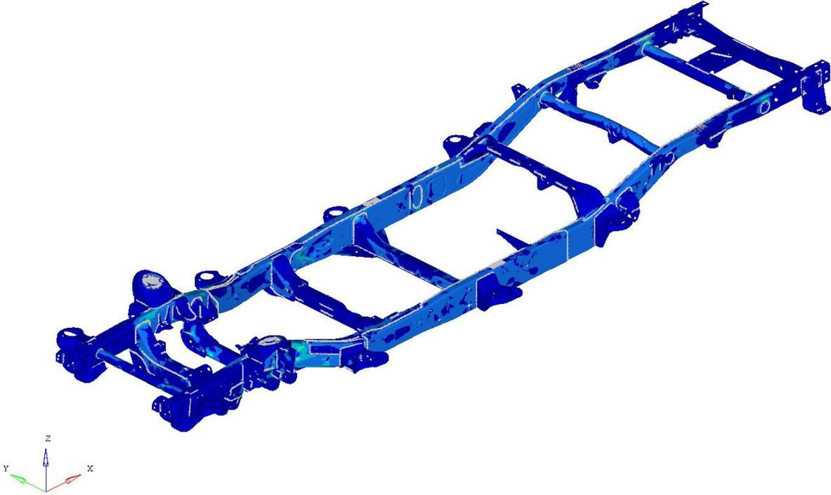
Figure A-14: Semi-manual TWB result: Von Mises stress for torsion LC
