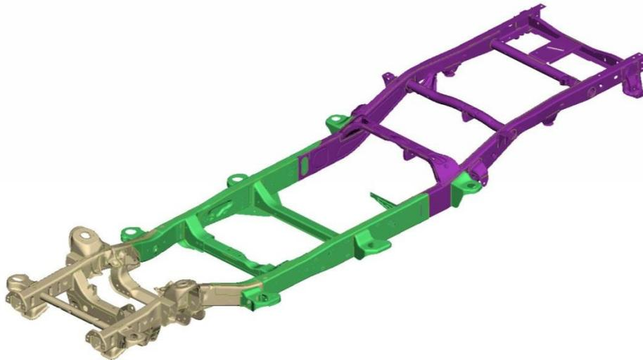
Figure 2-2: FE Model of Chevrolet Silverado 1500, Separated into Sections
