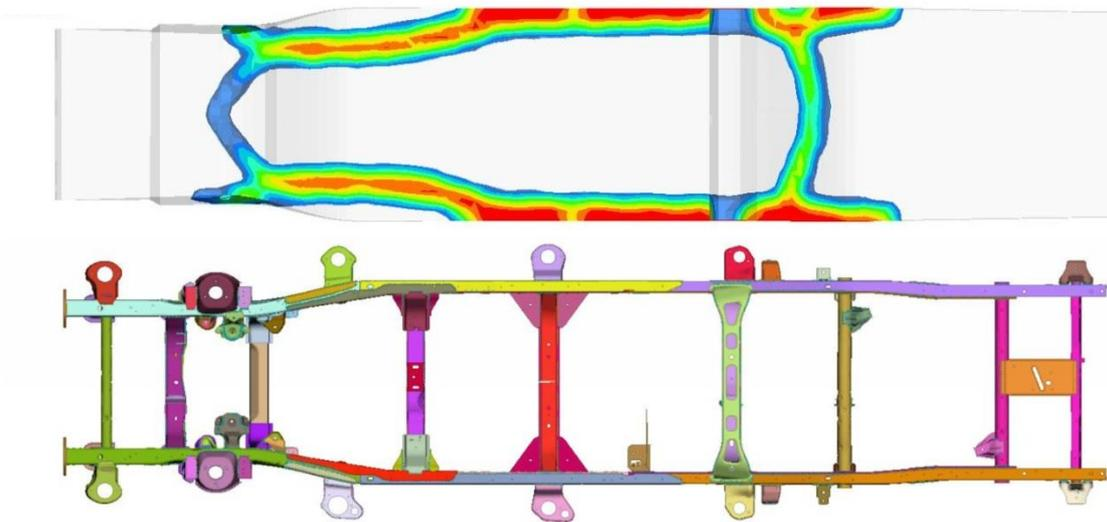
Figure 6-4: Comparison between the actual baseline model and the topological result
