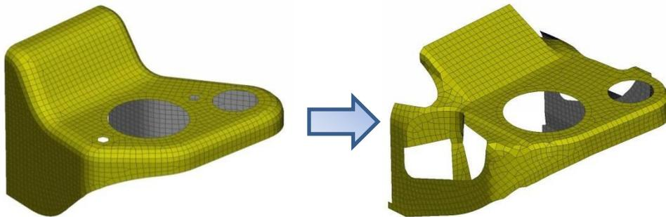
Figure 8-4: Changes being made from baseline model to the optimized result
