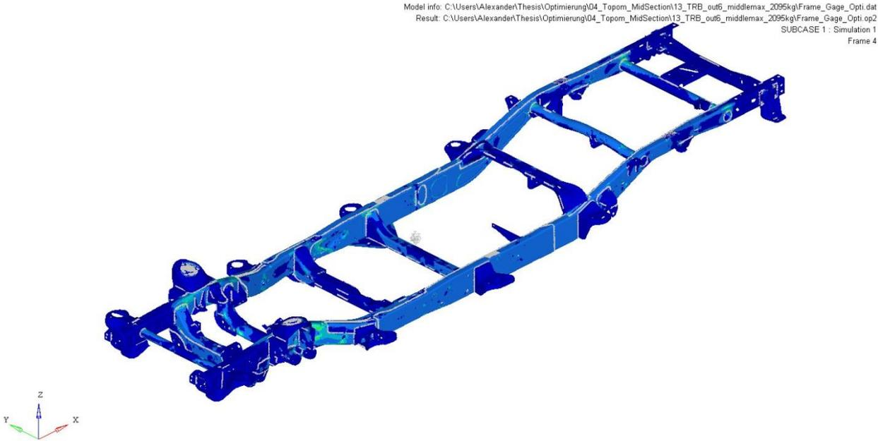
Figure A-16: Semi-manual TRB result: Von Mises stress for torsion LC
