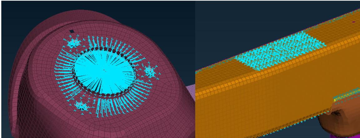
Figure 5-6: RBE 2 for application of force (left) and single point constraint (right)
