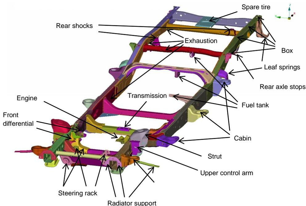
Figure 6-1: Overview of every module connected to the frame
