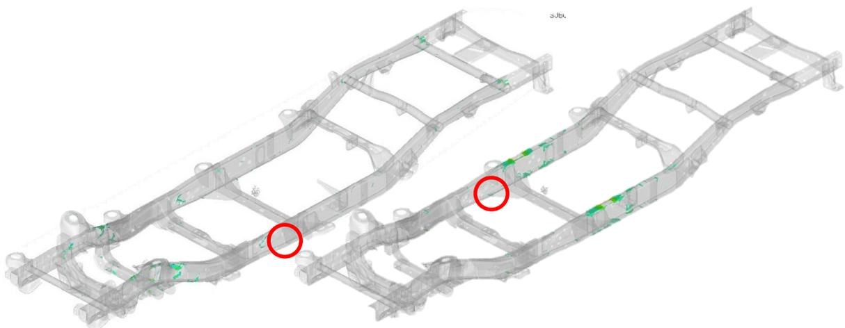
Figure 6-40: Semi-manual TRB: Von Mises stresses over 25 MPa
