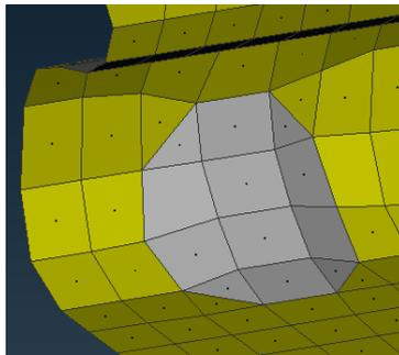
Figure 5-4: Finished FE model of a notch
