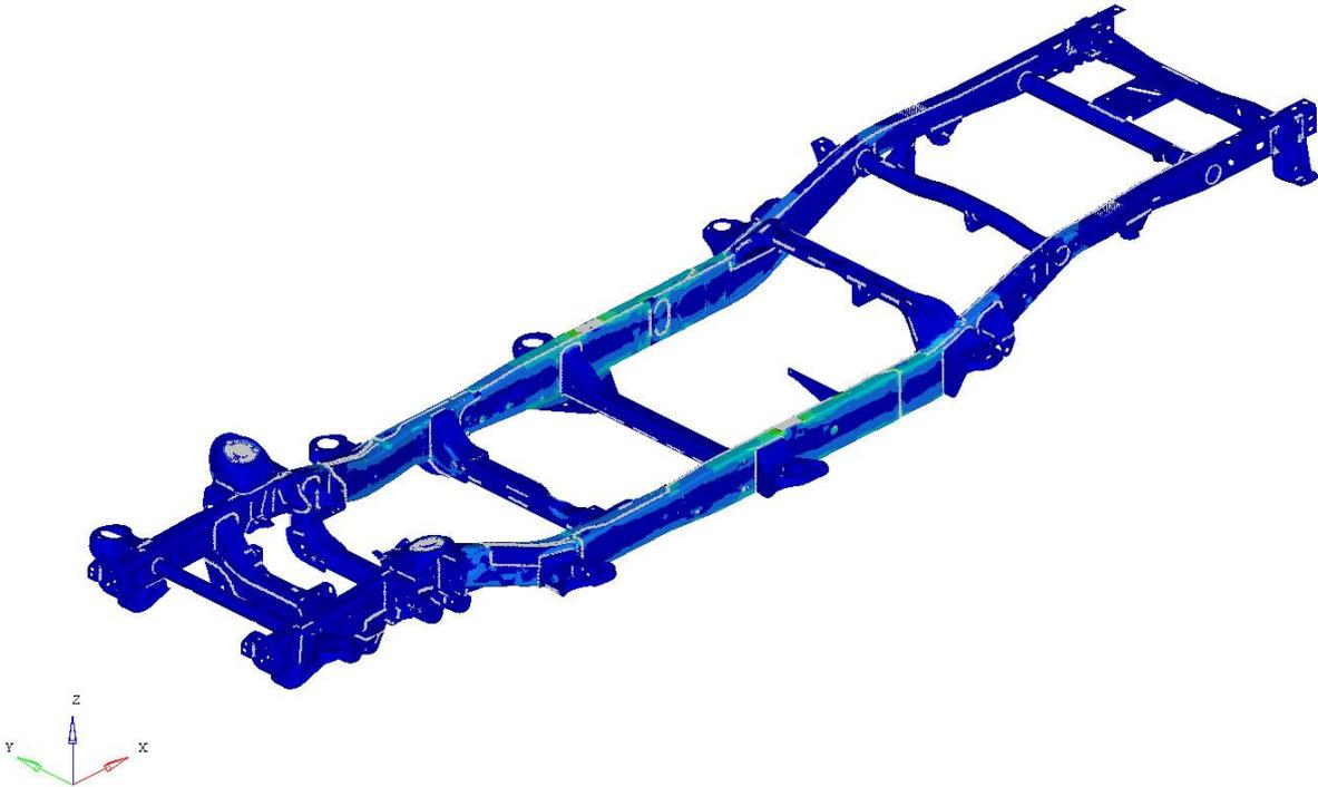
Figure A-13: Semi-manual TWB result: Von Mises stress for bending LC
