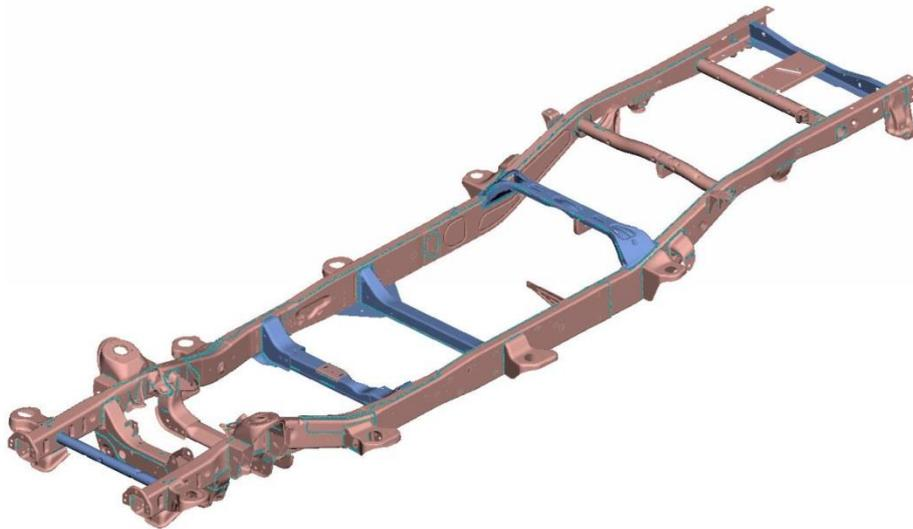
Figure 6-12: Selected parts for material optimization
