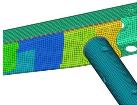
Figure 4-4: Topometry example for the frame
