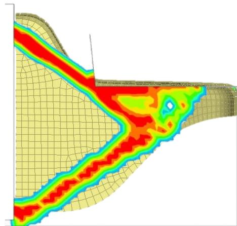
Figure 8-8: Merged side view of baseline model and topology result
