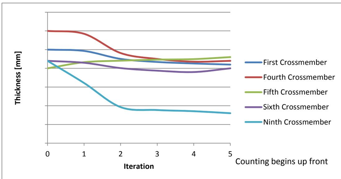
Figure 6-15: Material optimization: Thickness development of crossmembers
