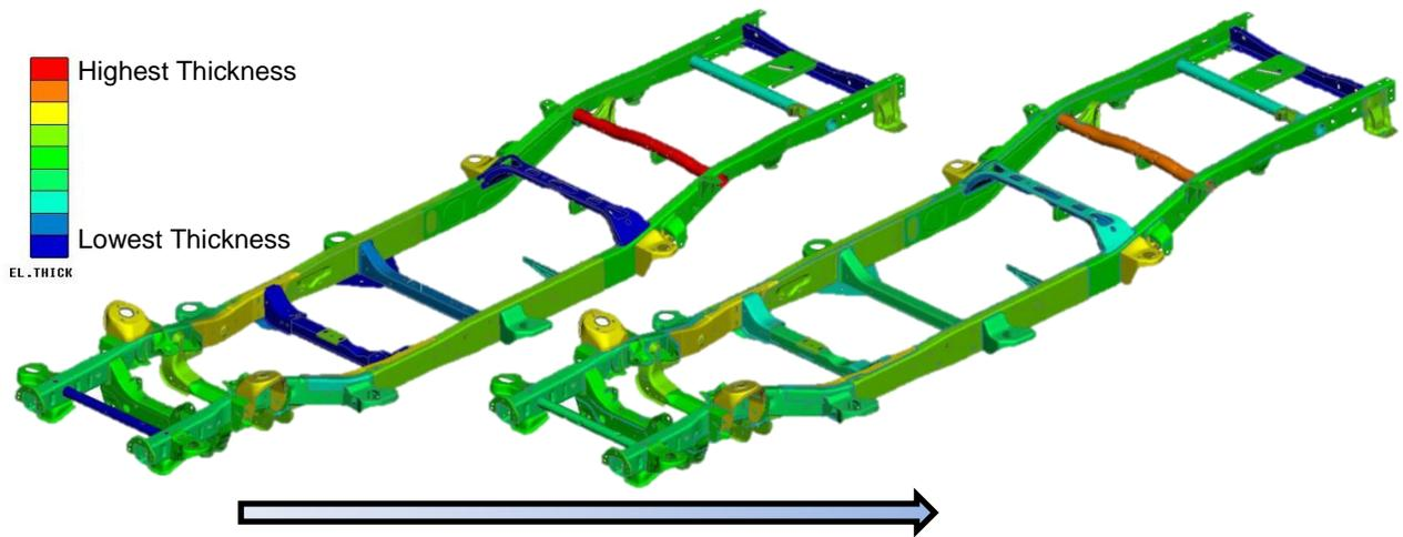
Figure 6-16: Thickness development from gauge optimization to material optimization
