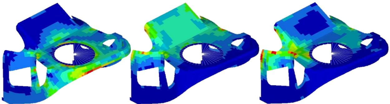
Figure 8-11: Von Mises stresses for: LC1, LC 2, and LC 3
