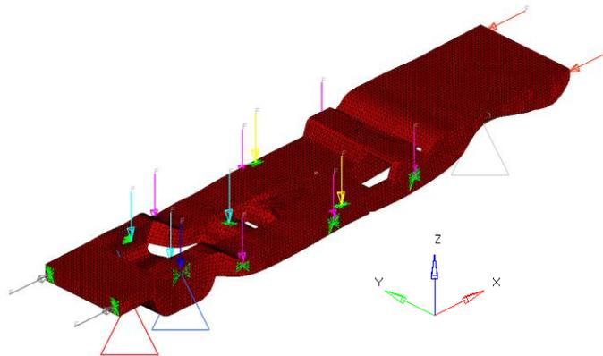
Figure 8-2: Overview of every Load and SPC applied on the model
