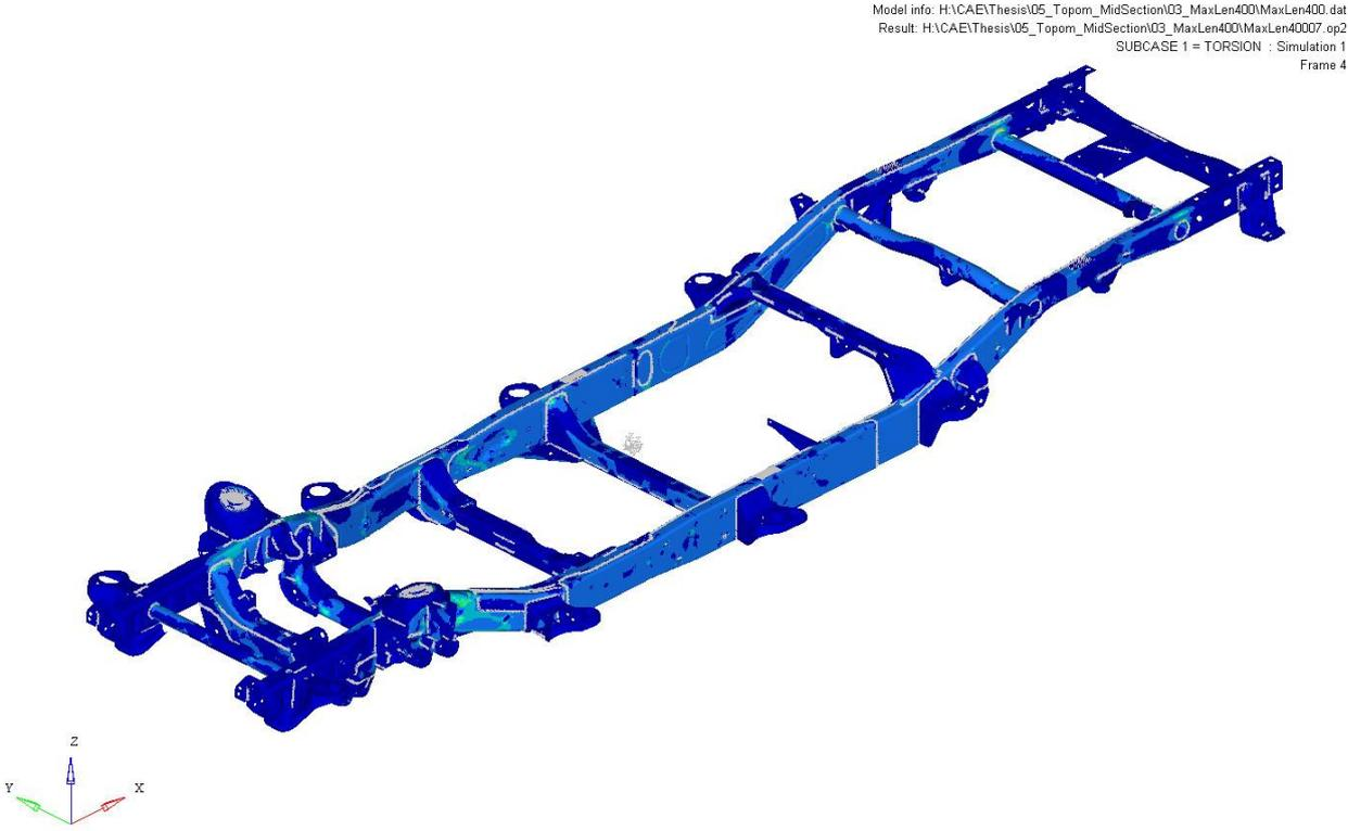
Figure A-12: TWB 400 mm width result: Von Mises stress for torsion LC
