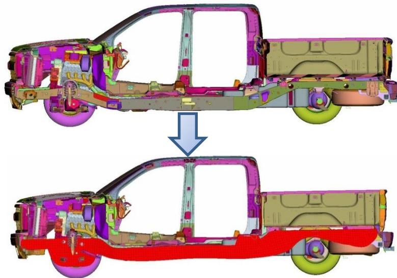
Figure 8-1: Analysis the structure to create an installation space model
