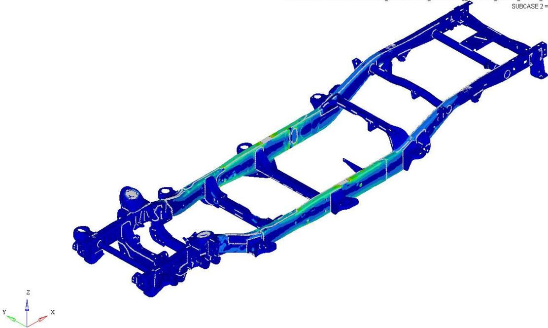
Figure A-1: Baseline result: Von Mises stress for bending LC
