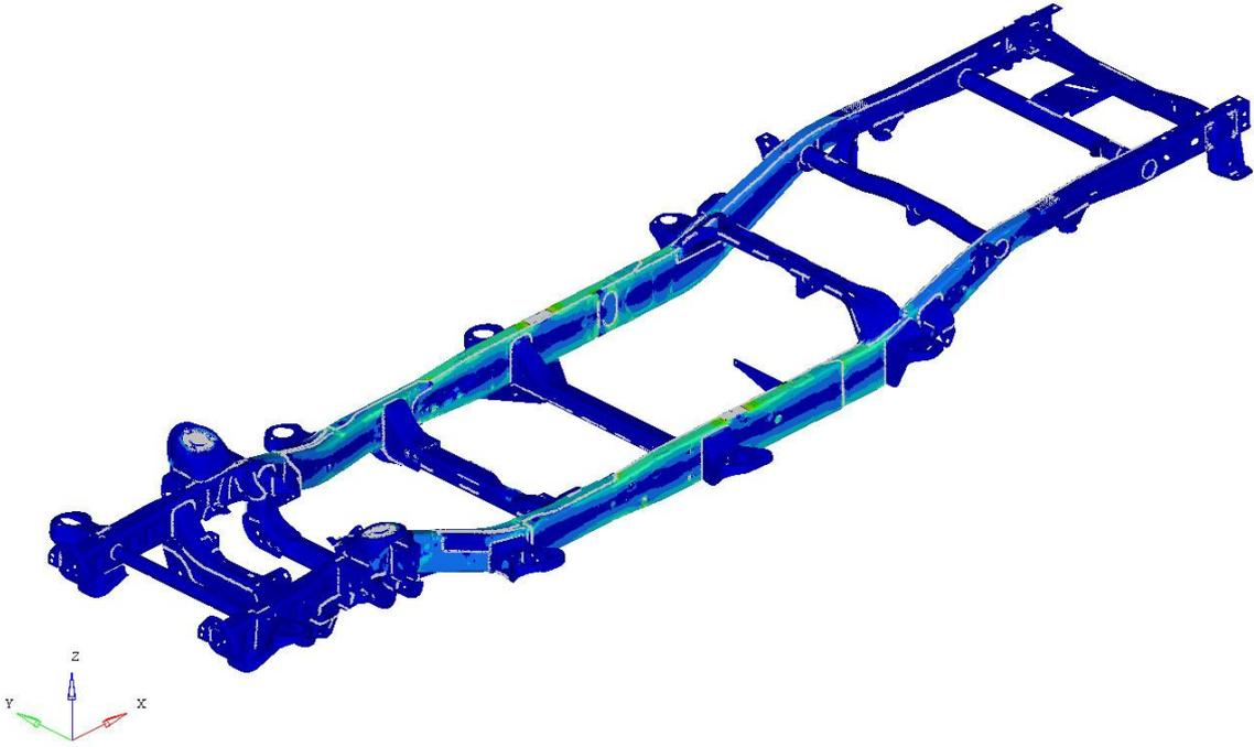
Figure A-5: Aluminum crossmembers result: Von Mises stress for bending LC
