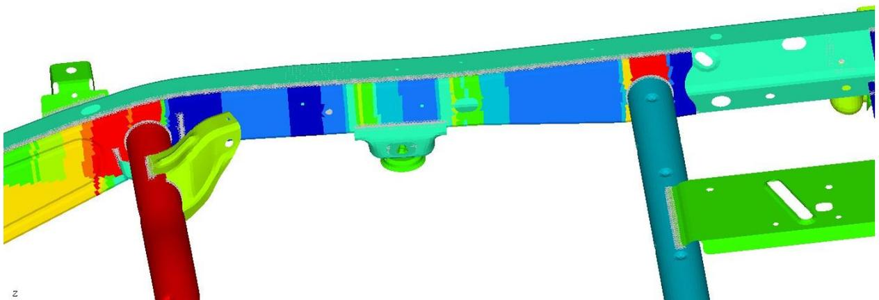
Figure 6-26: Topometry optimization results for the rear section
