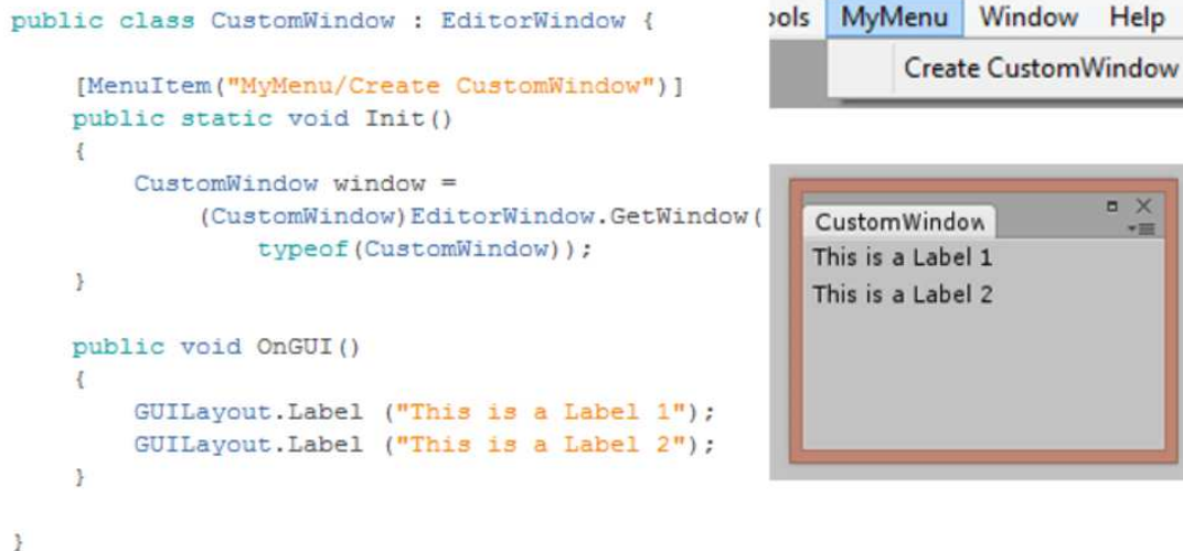
Figure 4.9 Example of EditorWindow class: CustomWindow script (left), creation of window through the static function Init (right above), GUI of window based on the OnGUI function (right below).
