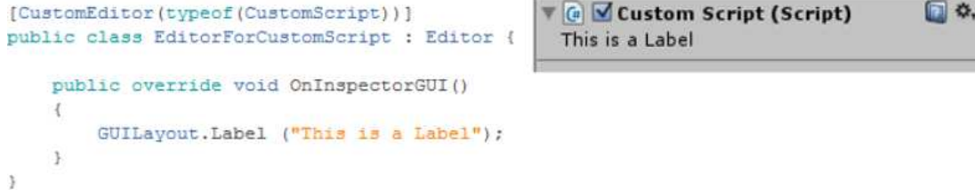
Figure 4.7 Example of EditorForCustomScript C# script (left) and its custom inspector view (right) for CustomScript . Notice there is different with default view of script in figure 4.6
