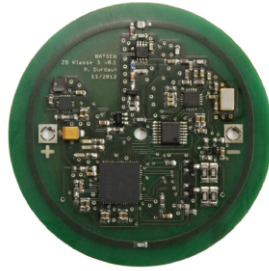
Figure 2.3.: Wireless cellular sensors with microcontroller, which are suitable to be integrated in large lithium iron phosphate round cells. Results of the project BATSEN at HAW.
