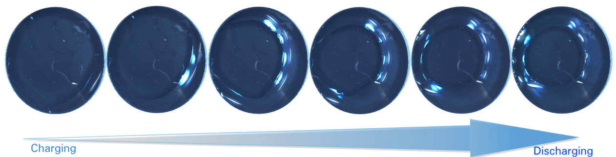
Figure A.3.: Gas bubbles on cathode (measurement series 17)
