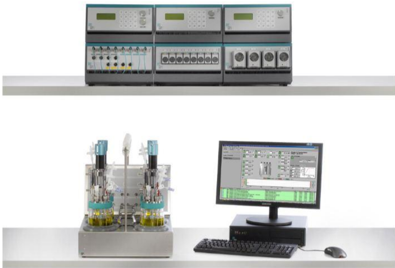
Figure 2-4: DASGIP bioreactor system. On top, gassing, temperature, pH, stirring, and pump modules are displayed. These are controllable in remote mode with the DASGIP software on a linked PC. The bioreactors are placed in a container and are connected to PC (bottom) and modules. Images were retrieved from www.eppendorf.com and were adapted.
