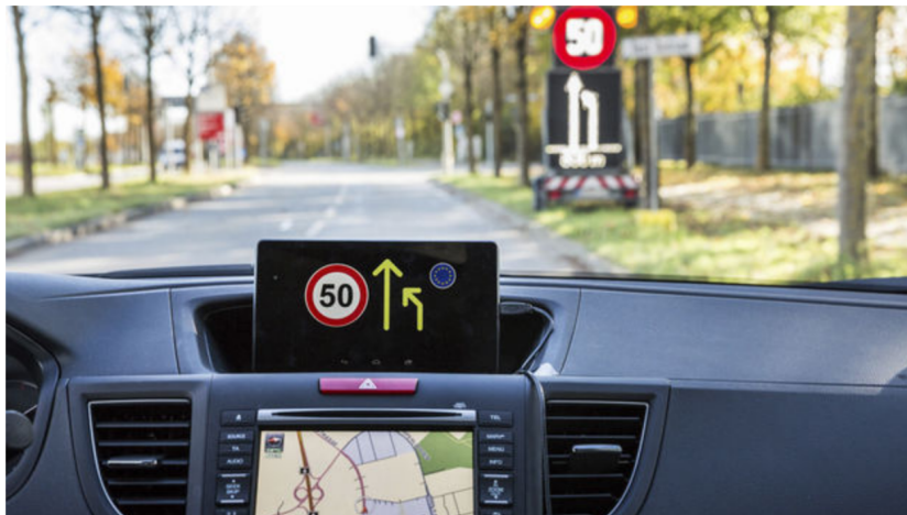
Figure 2.2.2-I: HID for driver assistance services. Source: NXP Semiconductors
