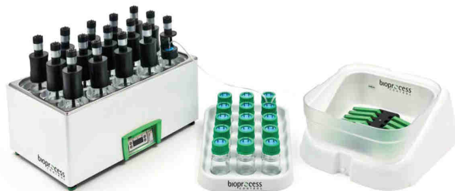
Abb.3-5-1: Automatic Methan Potential Test System (AMPTS II). [29]
