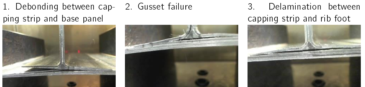
Figure 5.2: Three occurring failure types of preliminary testing of the T-Pull-specimen
