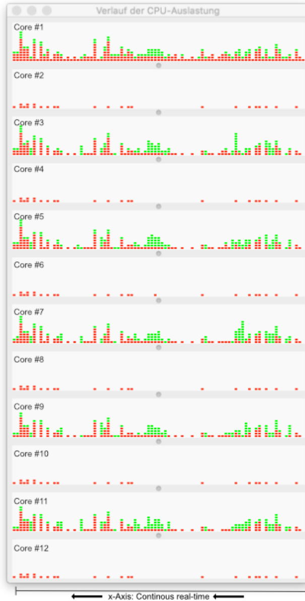
Figure 5.13: CPU load during consecutive runs of AgentShadowing benchmark on Mono. X-axis shows continuous time, while y-axis displays percentage of cpu usage per core from 0 to 100.
