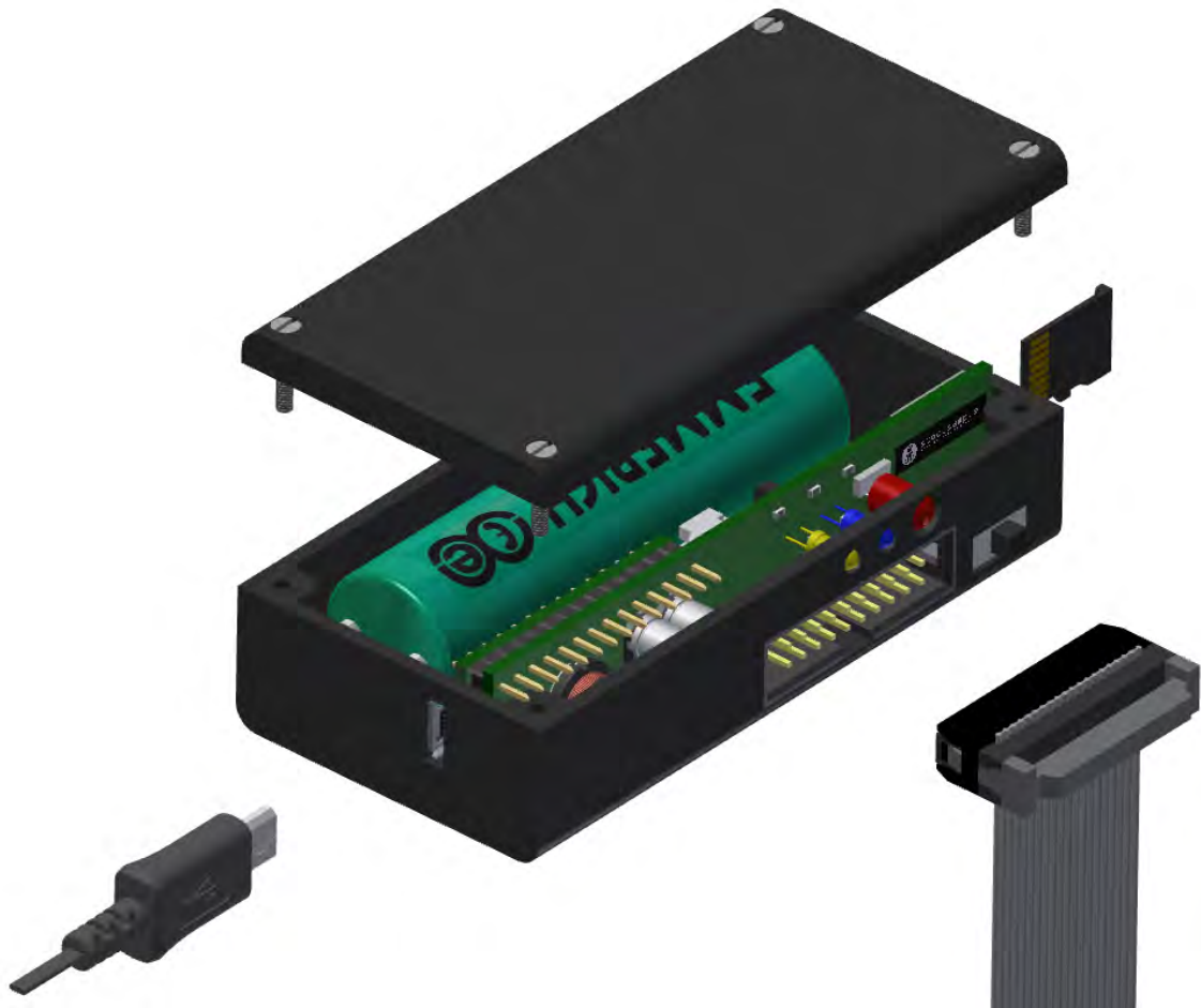
Figure 4.1: Rendering of the data logging unit with Micro-USB, microSD, and 20-pin flat cable sensor connector.
