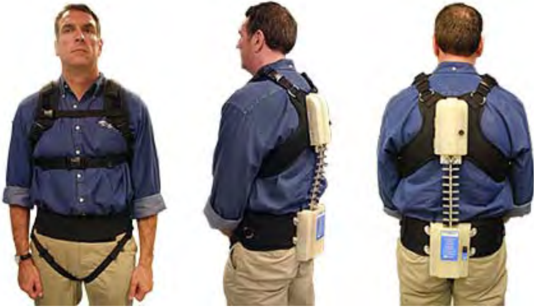
Figure 3.2: Body-based mechanical motion tracking of the spine: The AccuPath Industrial Lumbar Motion Monitor [47].
