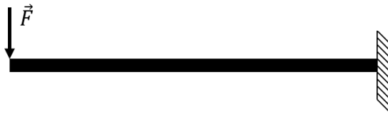
Figure 5.9: Schematic model of a cantilever
