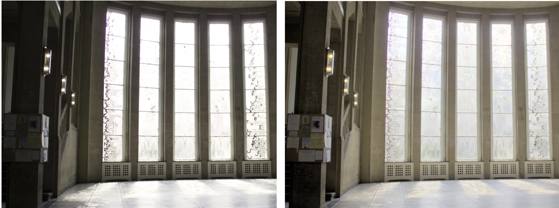
Figure 1.1: Left: a standard photo, as captured by a modern digital camera. Right: an HDR photo generated by combining photos of various exposures, tone mapped using the method described in this thesis. Note that in the image on the right, there are details visible in the bright areas that are clipped to white in the left image.
