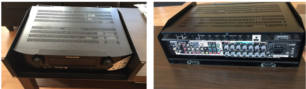
Figure 21: Custom made rack mount for the AV receiver
