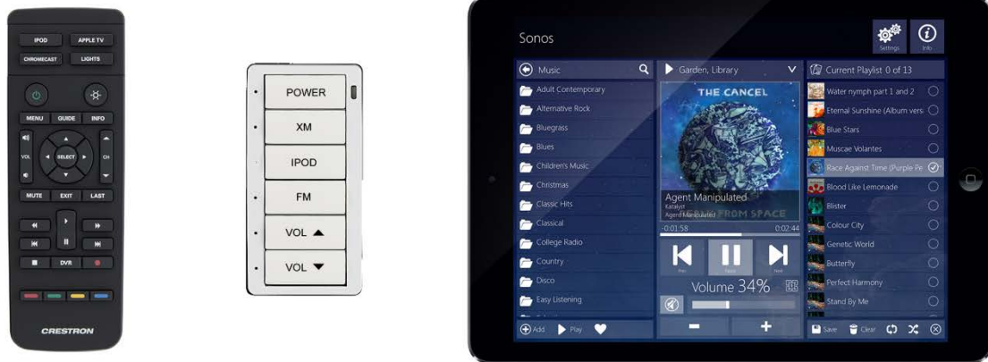
Figure 14: Control Devices: Crestron remote, keypad and Apple iPad with a Crestron GUI
