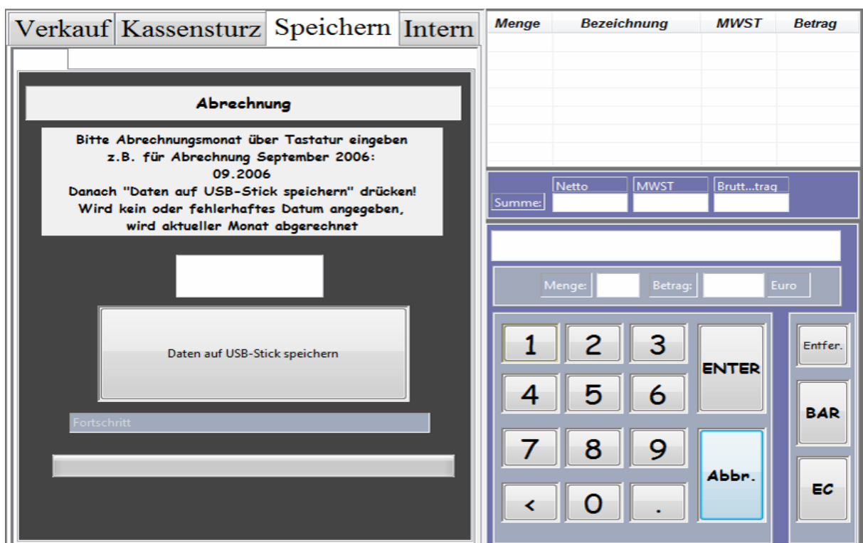
Figure 5-12: The tab “Speichern” for external storage on USB-stick is chosen
