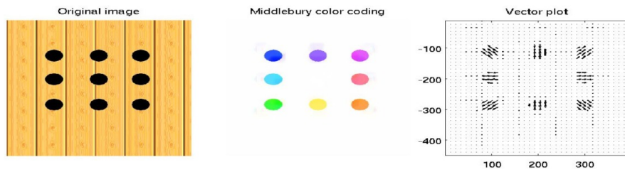
Figure 4.7.: Vector plot and color coding represent the direction of movement of circles with background.
