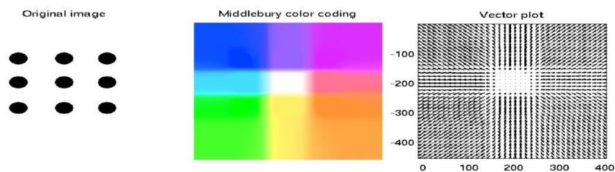
Figure 4.6.: Vector plot and color coding represent the direction of movement of circles without background.
