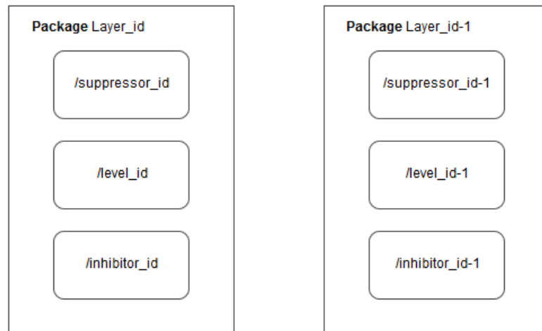
Figure 6.7: ROS File System Structure of Subsumption Architecture
