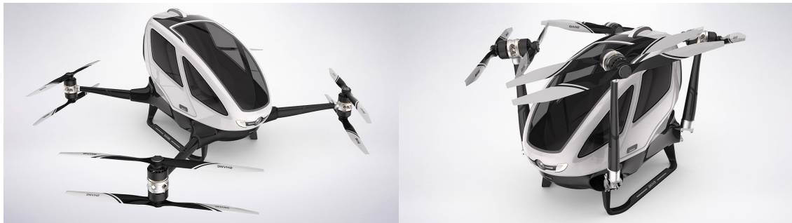
Figure 5: The Ehang 184. The propellers fold to fit in parking spots (right image)
