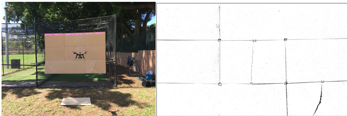
Figure 18: Test picture for crack detection
