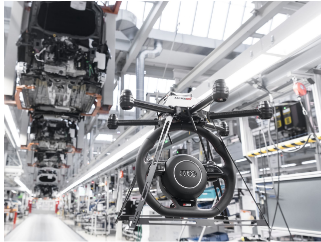
Figure 2: Transportation of a wheel for intralogistics by the UAV [1]
