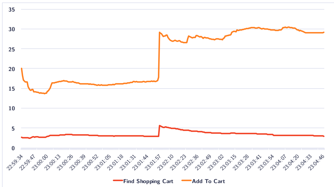
Figure 7.5: Response times in milliseconds of methods in the order service during the second load test case on the conventional system.
