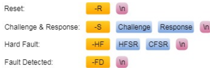
Figure 4.3.: UART frame format for Client-to-Host messages
