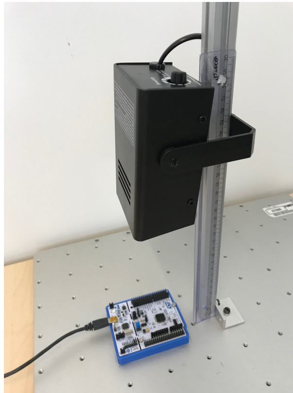
Figure 3.7.: Setup for experiments with xenon strobe light
