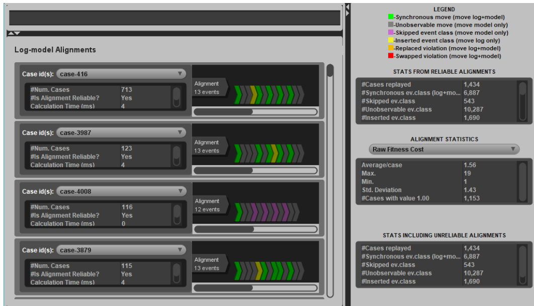
Figure A.16.: 'Project Alignment to Log' of the 'Replay a Log on Petri Net for Conformance Analysis' plug-in applied to the environmental permit application process event log and model.
