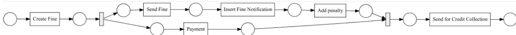
Figure 4.7.: Petri net mined by applying the 'Mine with Inductive visual Miner' plug-in
