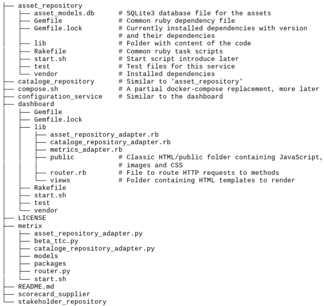
Figure 5.1: Overview of the projectstructure
