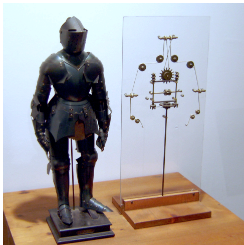
Fig. 2.1: Model of Da Vinci's humanoid robot with mechanisms inside (Da Vinci, 2005)
