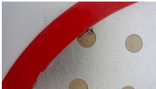
Fig. 7.3: Damage inside the static port area; need for further investigation (LHT, 2018)
