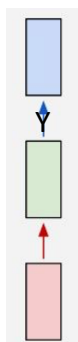
Fig. 4.11: Vanilla RNN; X (red) represents input, Y (blue) represents output, hidden neuron (green) represents the core of the RNN (see Li, et al., 2017)
