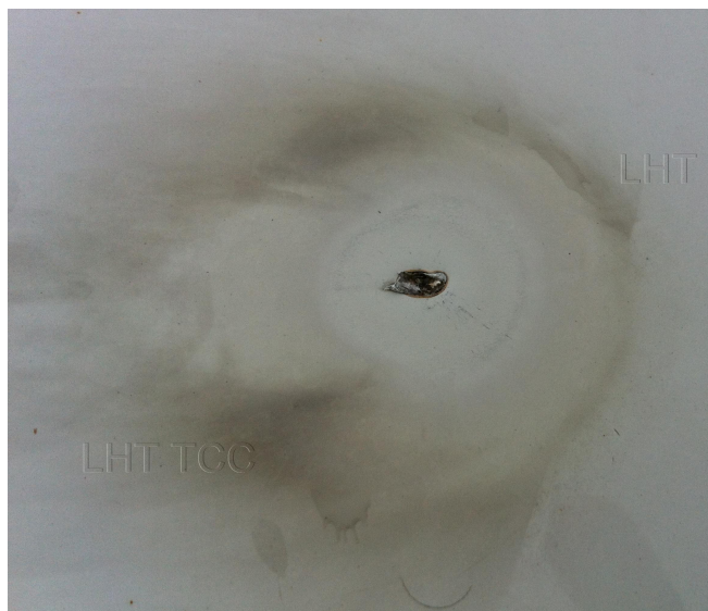
Fig. 7.1: Lightning strike to the skin with a burn mark (LHT, 2018)
