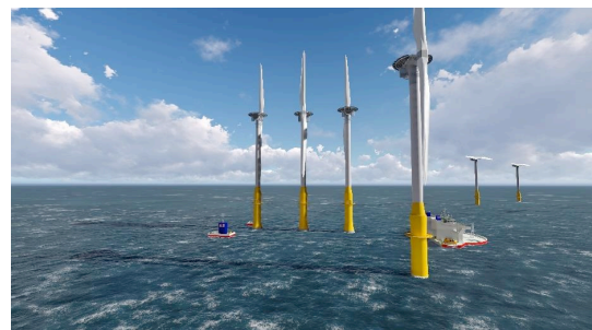
(3) Seawind 6.2 MW turbine with helicopter landing platform and installation procedure (illustration)
