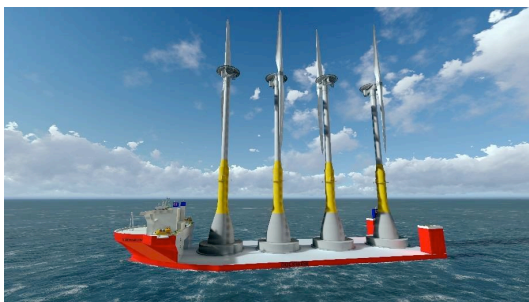
(3) Seawind 6.2 MW turbine with helicopter landing platform and installation procedure (illustration)
