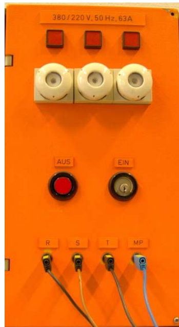
Figure 5.4 Power supply 380 V
